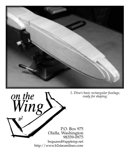
As mentioned in last month's column, construction of the Diva airframe has been completed for some time. As we receive so many questions about how to achieve a smooth aerodynamic fuselage from basic sheet and block construction, this month's column is primarily devoted to explaining how we accomplish that task. We've also included some photos of the completed framework just prior to painting and covering.
