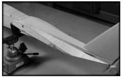
3. Another view of the wing-fuselage fillet. The rudder pushrod exits the fuselage just above the fillet.
