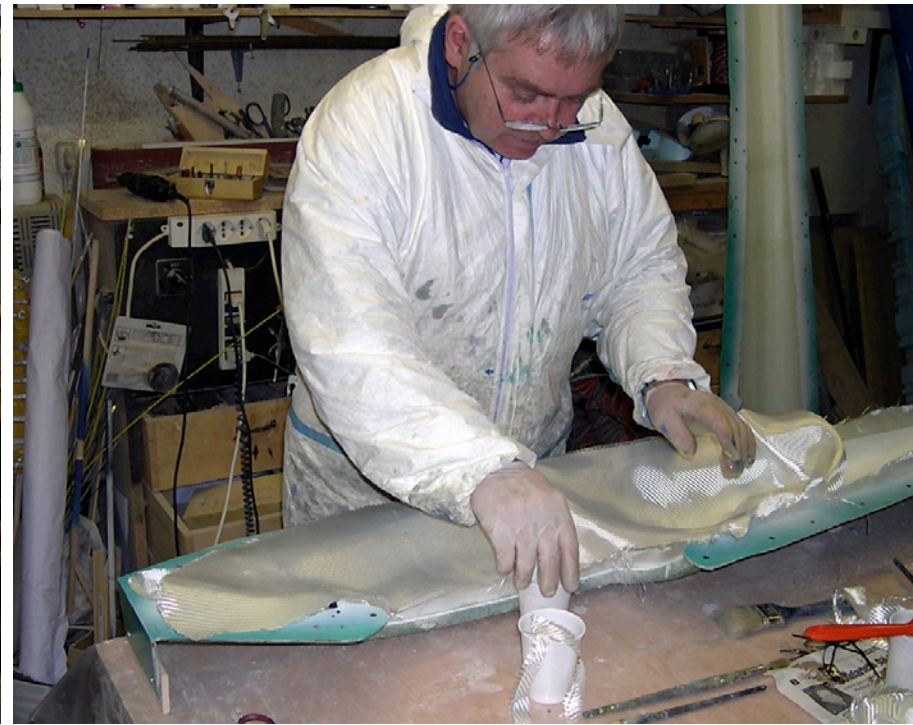
Left: One half of the fuselage mold is set up on a sturdy flat table. Right: The first layer of glass goes into a mold.
