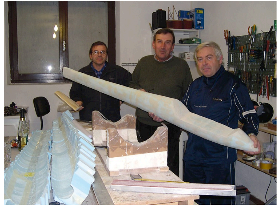
Left: Well into making the fuselage plug. Right: The finished fuselage plug. The author stands in the middle.
