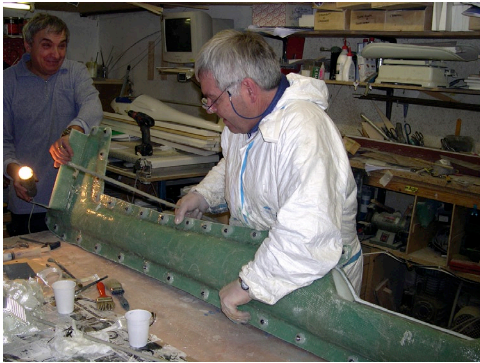
Left: One half of the fuselage mold is set up on a sturdy flat table. Right: The first layer of glass goes into a mold.
