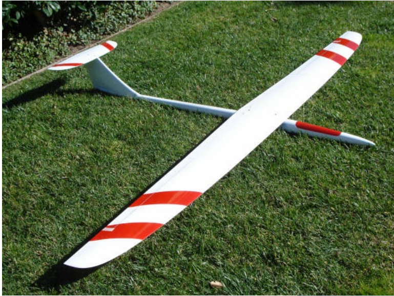
Hybrid Kinetic 100 Fuselage is Version 1, wing and stabilizer are Version 2. The revised wing and stab section came from Delft in Germany.
