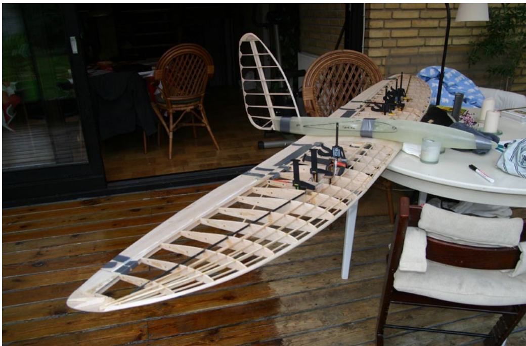
Construction of the wing joiner boxes showing the carbon fiber wrap, and a rough test fitting of the various parts just to get an impression of the size of the R-2.
