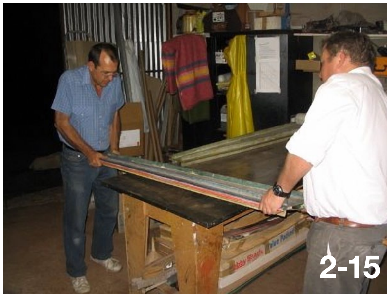
2-15: A week later the bolts and clamps are removed and the molds twisted slightly to loosen the wing from the molds.
