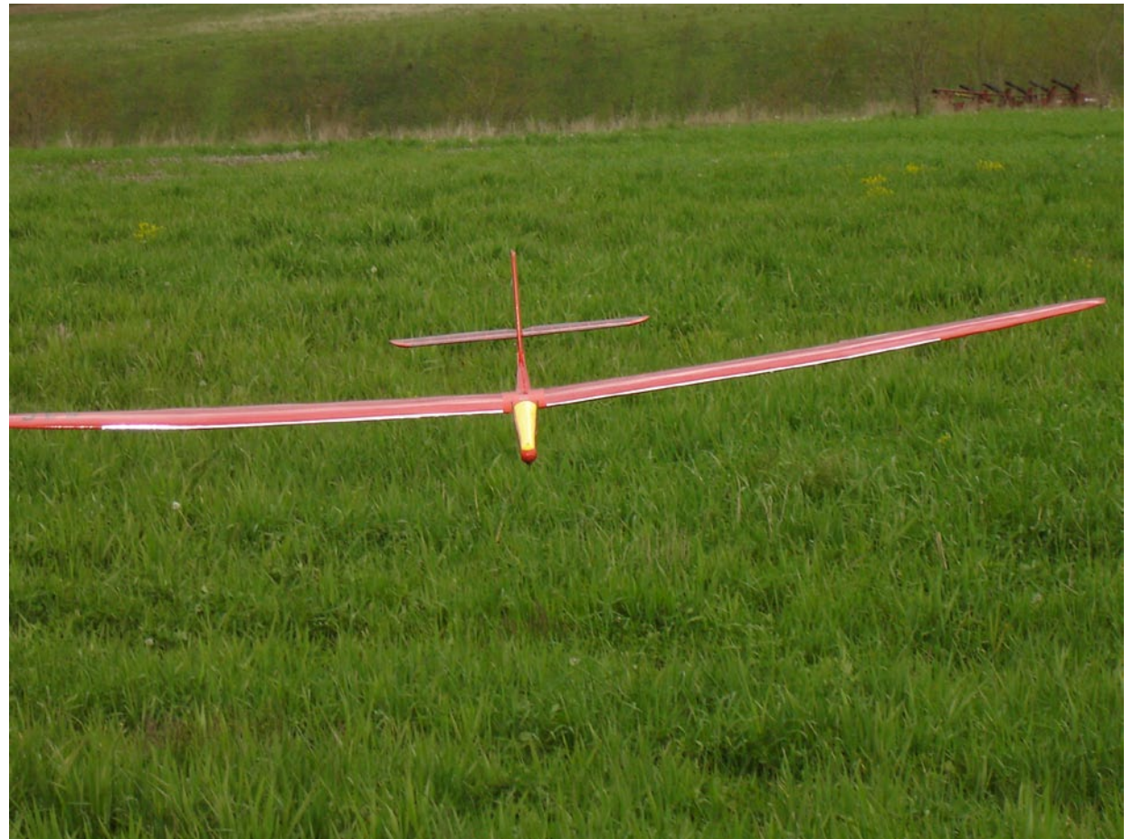
Landing the Apache can be a challenge. The small cross section makes it hard to judge distance and speed. Due to the high grass I normally retract the flaps just before touchdown.
