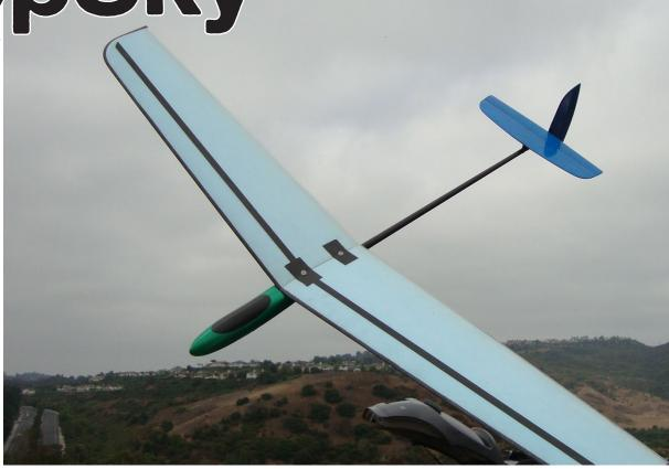
Technical Data: Wingspan: 1000mm (39.3 in.) Wing airfoil: AG03 AUW: 135g (4.5 oz)
