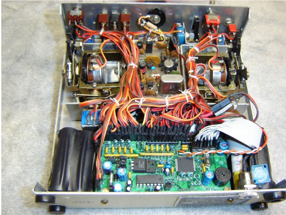
The Version 5.0 encoder is at the bottom center of the case. The two battery packs are placed each side. Connectors along the topside of the encoder are for trims and controls. The 3-pin Deans connector at the right side disconnects the battery. In the center, just above the encoder, is the Ace RF deck. The LCD display is underneath the encoder with the connecting ribbon cable visible at the right side of the encoder.
