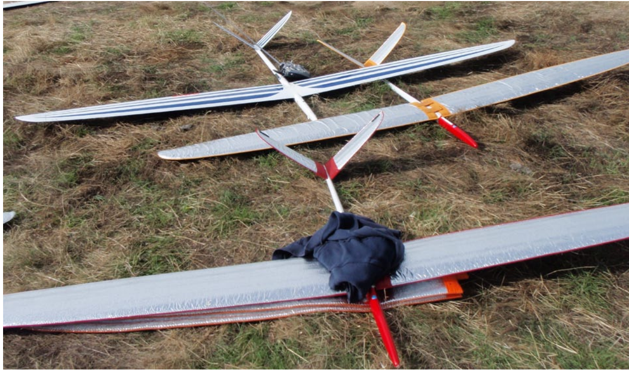
A selection of 'ships specifically designed for the three F3B tasks - Duration, Distance and Speed. Because of the relatively low weight given to landing points, V-tails are more popular here than in the usual thermal duration contest.
