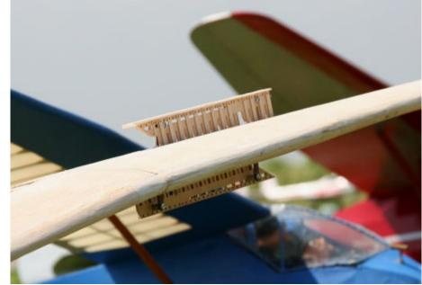
The intricate "double comb" airbrakes.
