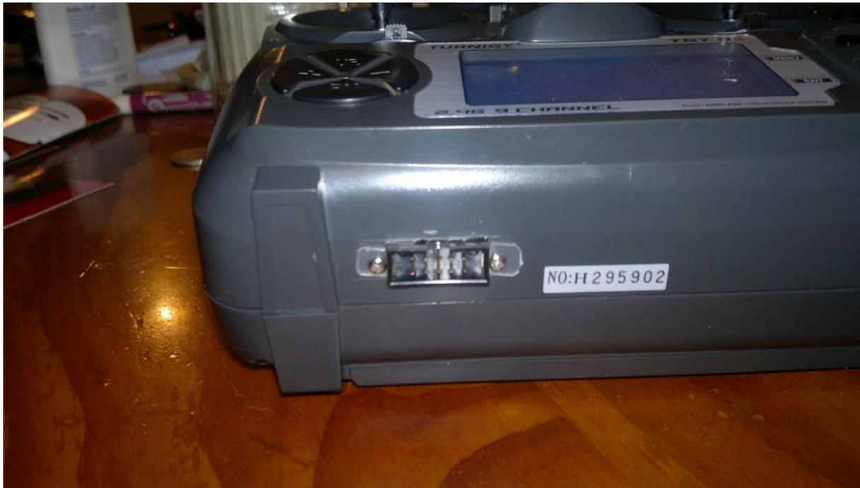
*How I have installed the IDC female header. The programmer is joined to this via a cable with male IDC headers at each end.*
