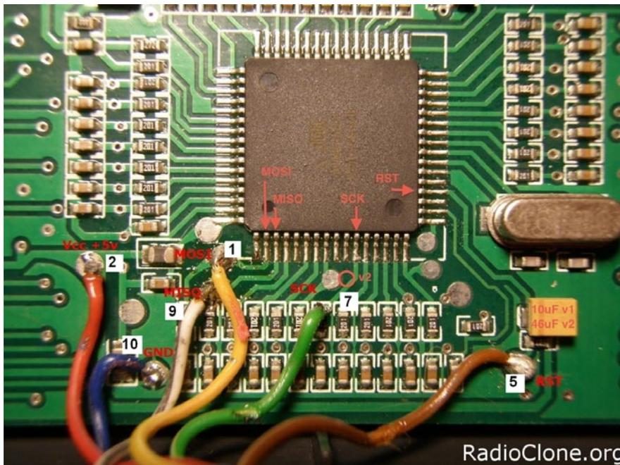
This image shows the pads and what wires are soldered to them. Numbers for the ribbon cable start with 1 on the pink/red side through to 10 at the other side. Note the red circle for SCK, the radio in the image is version 1 and this wire is soldered to the resistor. All radios sold now are version 2 and there is a pad where the circle is that this wire is soldered to.
