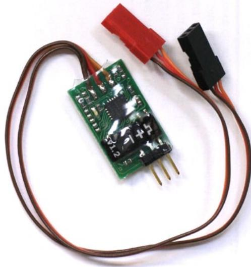
set is often not used on a sailplane. The device is switched off for most of the flight - we do not want the rudder wagging on tow, or when climbing out under electric motor power. After the sailplane enters cruise mode, and when switched on from the transmitter, it indicates rising air by gently wagging the rudder side-to-side, sensing a decrease in atmospheric pressure to detect lift.
