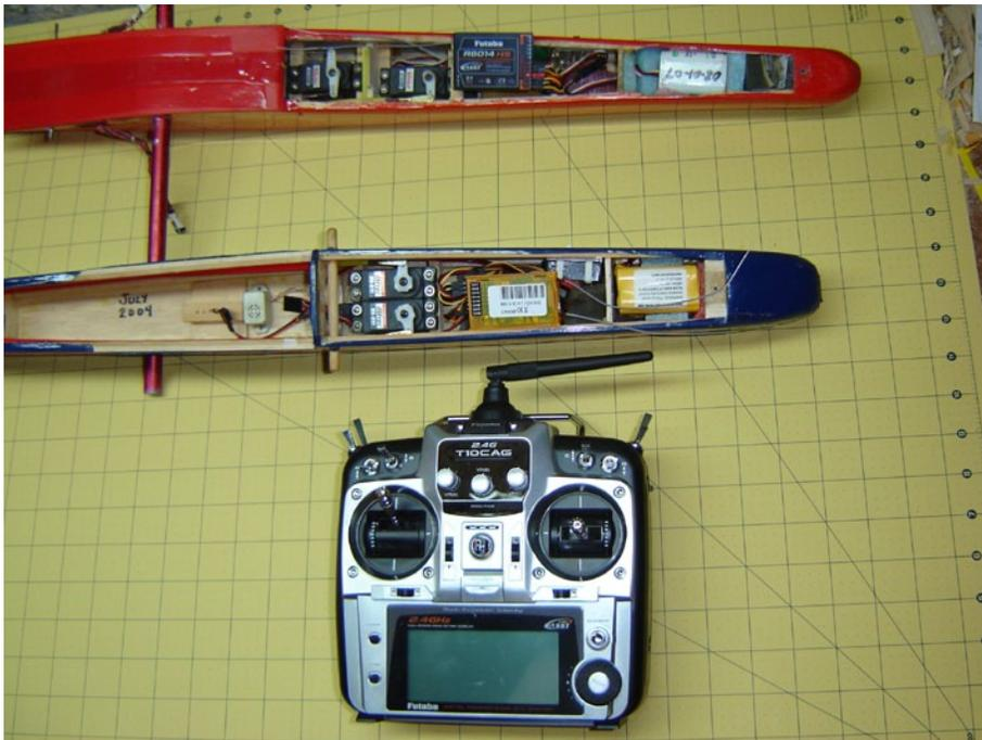
The Orange receiver fits a typical fuselage radio room in the same manner as the Futaba. Coaxial cable antennas are installed at 90 degrees from each other and battery and servo connections are the same. The Orange receiver requires that the 10CG transmitter be placed in 8-channel mode with the fail-safe feature disabled to prevent servo jitter.
