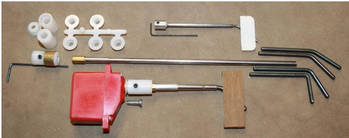
*The new G2 System with the coupler engineered to control unwanted rotation and allow a sliding fit with the hex-ended drive shafts.*
