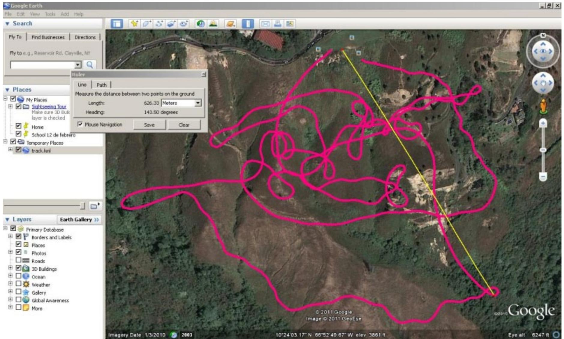
*After downloading data from the Canmore GT-730FL-S USB GPS Tracker Stick Data Logger, the flight track can be plotted on Google Earth. Distances can then be measured directly on-screen.*
