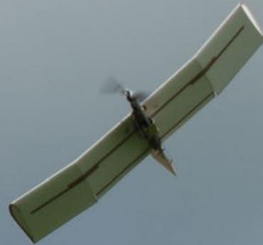
*A foamie electric "plank" for thermal flying*
