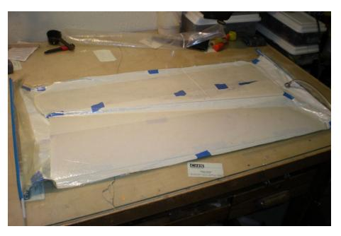
The wings in the shucks being pressed and curing.
