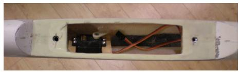
Left: The wing seat filled in and shaped with the wing. Above: The wing bolt blind nuts installed and the elevator servo.
