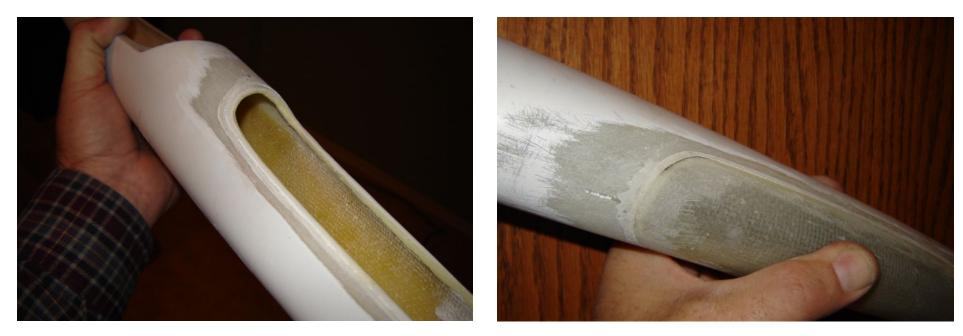
These photos show the new epoxy added to the fuselage to make a seat for the canopy.
