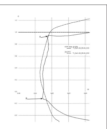
Figure 1. Using an arbitrary value of CL at low-speed end, e.g. 1.0 (heavy line), would have given an unrealistically poor rating to some foils, as with E374 in this instance. Accordingly I used 1/L/Dmax for all foils, as measure of high-CL drag. For both foils shown, L/Dmax would be near point A. Note how E374 has higher drag everywhere except at two small peaks, A and B. 2. Author-generated Foils:
