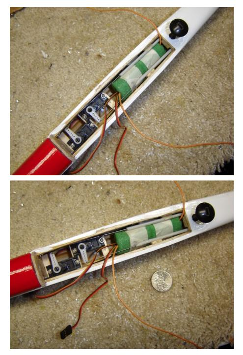
The two orange wires are the Scout transmitter antennas. They should be taped to the bottom of the wing in a "V" pattern for best reception on the ground.
