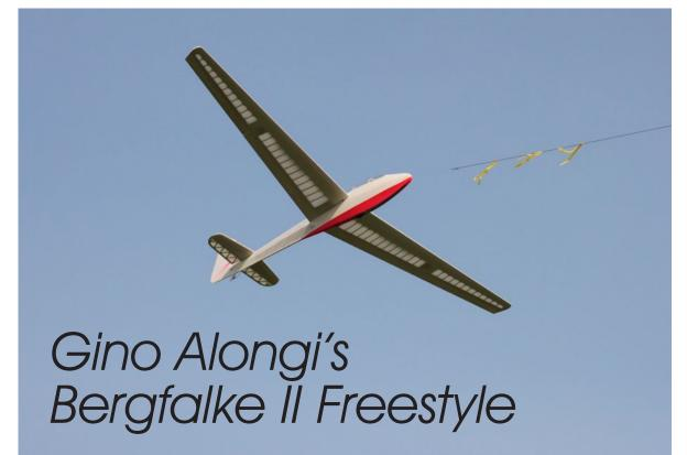
A 1:4 semi-scale model of the circa 1955 full size glider designed with AutoCAD, Profili2, and XFLR5 and built using laser-cut parts. Features include RDS aileron control, Oratex covering, removable stabilizer and pre-tensioned hooks for mounting of the wings. Capable of aerotow and slope flight.
