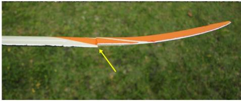
Above: 1° was imparted into the wing tip using epoxy to reglue the joint.
