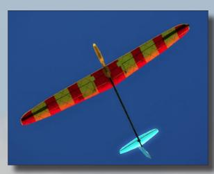
Front cover: Phil Pearson captured this image of Ken Lies' DLG at a contest in Pasco Washington last year. Ken built the airframe using a Zone wing. Valspar paints for coloring; red color down first then light layer of yellow over the entire bottom mylar. The tops are solid red which gives the thinner flaperons the orange hue. Nikon D300S, ISO 200, 1/125 sec., f5.3, 230mm
