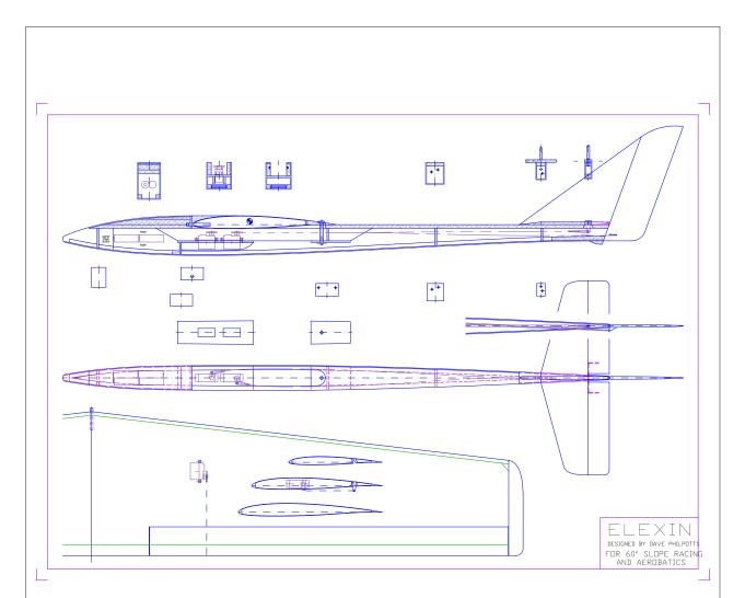
ELEXIN, designed by Dave Philpotts for 60" slope racing and aerobatics Full size PDF plans (34" x 44") are available from the web site of: Associação de Planadores Radiocontrolados de Belo Horizonte/MG <http://www.planabh.com.br/elexin.pdf>
