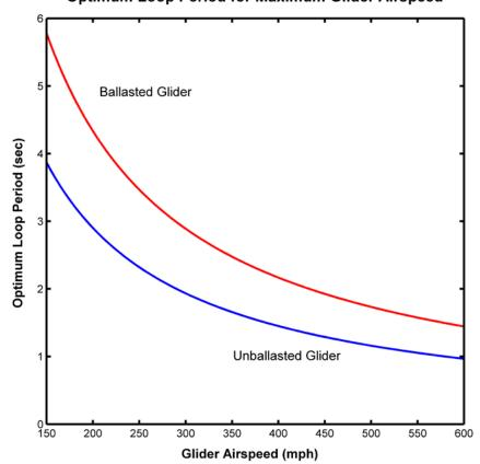
Figure 3. Optimum loop period  $t_{opt}$  required to achieve the maximum glider airspeed in a Rayleigh cycle plotted as a function of glider airspeed. Curves are shown for the unballasted ( $V_c = 45$  mph) and ballasted ( $V_c = 55$  mph) gliders. Ballast is around 50% of the unballasted glider weight.
