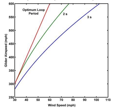
Glider Speed vs Wind Speed for Different Loop Periods
