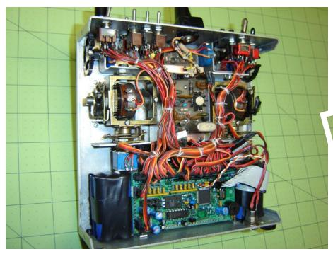
The ProLine case and sticks are a tight fit for the electronics. This requires very careful planning during installation of the various components. For example, the 8-cell NiCad battery is split into two 4-cell packs to fit either side of the encoder board. The Ace RF deck fit very well between the stick assemblies with the on-off switch underneath. The LCD screen is mounted to the inside of the case under the encoder board.
