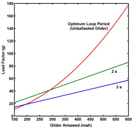
Figure 5. Load factor plotted as a function of glider airspeed and different loop periods for the unballasted glider ( $V_c = 45$ mph). Load factor is equal to the total acceleration of the glider in terms of the acceleration of gravity (g).
