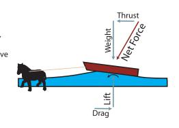
Figure 17: Flow similarity: Dissimilar forces in similar patterns make similar wave motions. © 2011 Philip Randolph
