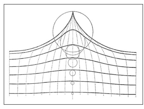
Figure 3: Horace Lamb's 1895 interpretation of von Gerstner's 1802 deep-water wave-circulation diagram As a wave passes, the water that makes it up moves in complete circles, that diminish with depth.
