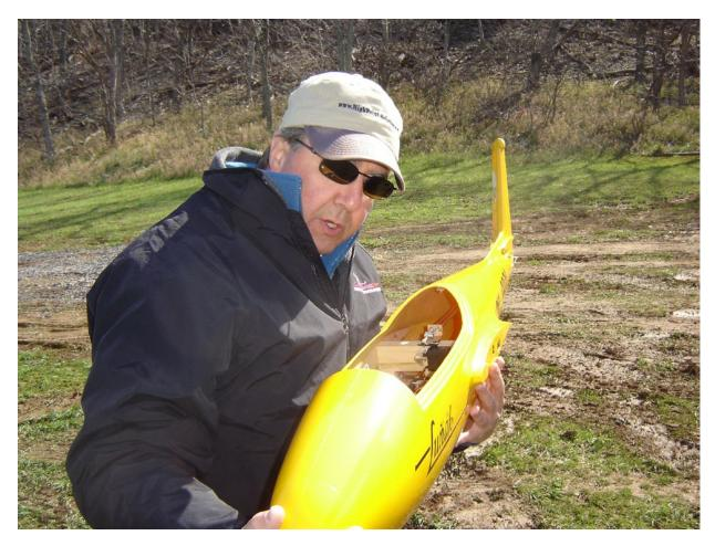
Above: Jim Dolly holds the Lunak fuselage as the elevator controls were checked out. It had two pushrods, one to each elevator half, joined to single ball link at the servo. Pushrod lengths were individually adjustable to set trim.
