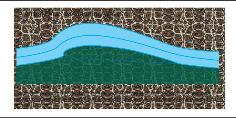
Figure 20A: Standing waves over airfoil shapes in a streambed. © 2011 Philip Randolph
