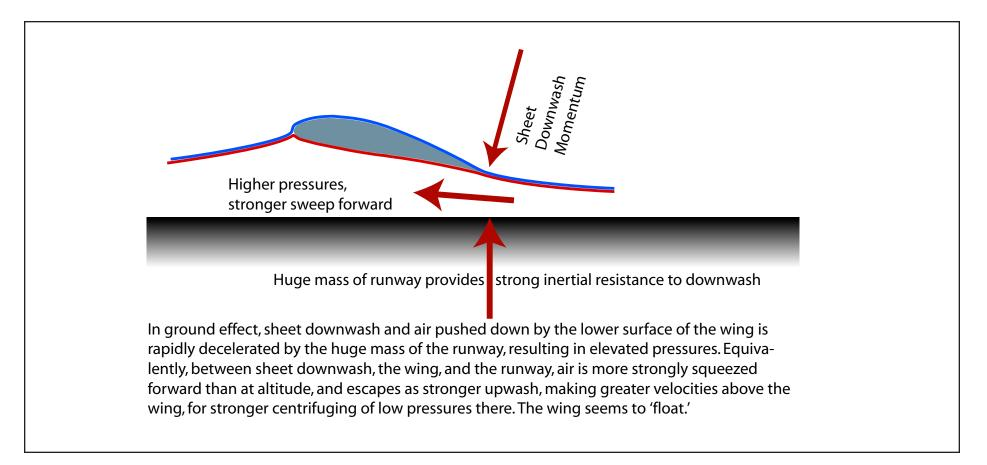
Figure 15B: Upwash, ground effect, lower energy recycling. © 2011 Philip Randolph
