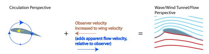
'Adding' a linear flow velocity to asymmetrical 'circulation' velocities makes an even more complex waveform, the wing wave. But flow and circulation velocities are inseparable. What we really change is the velocity of the observer.
