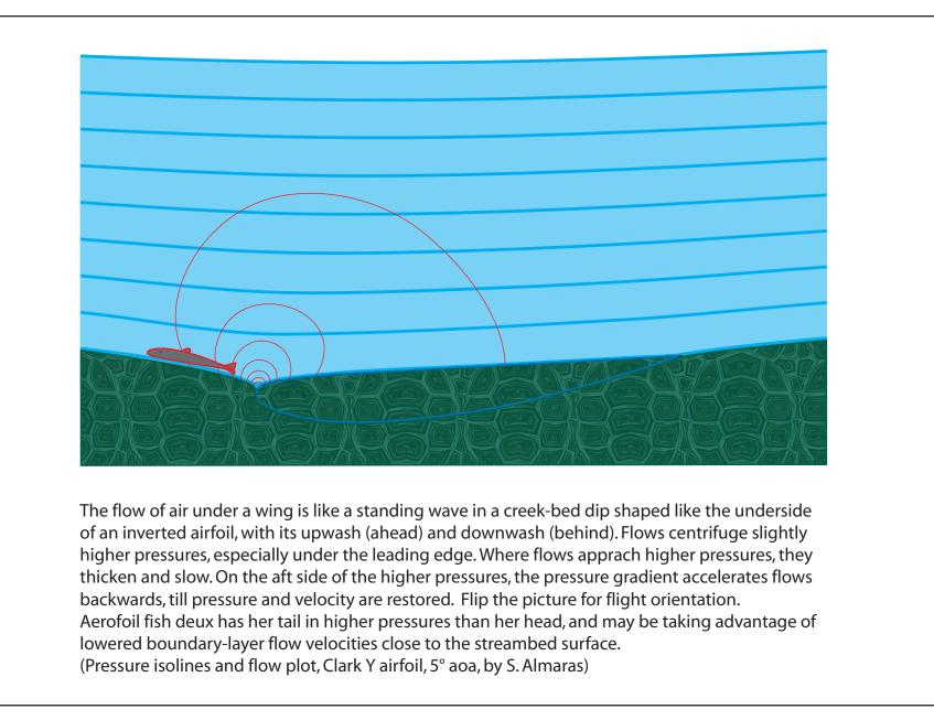
Figure 20C: Standing waves over airfoil shapes in a streambed. © 2011 Philip Randolph
