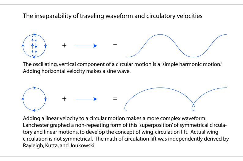
Figure 4A: The inseparability of waveform and circulatory velocities. © 2011 Philip Randolph
