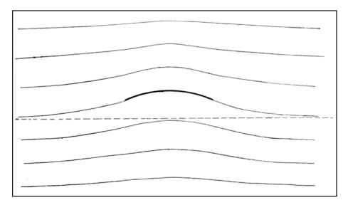
Figure 1: Lanchester's ;supporting wave' diagram, used in his 1894 presentation. He only applied such symmetry and perfect lift to infinitly long wings in inviscid (frictionless), incompressible fluids. The airfoil was curved to match the path of air, to avoid 'discontinuities' at leading and trailing edges, a requirement later known as the 'Kutta condition.' Flows over a subsonic wing in lift always show waveform, with upwash ahead rising to a crest, and downwash behind. © 2011 Philip Randolph
