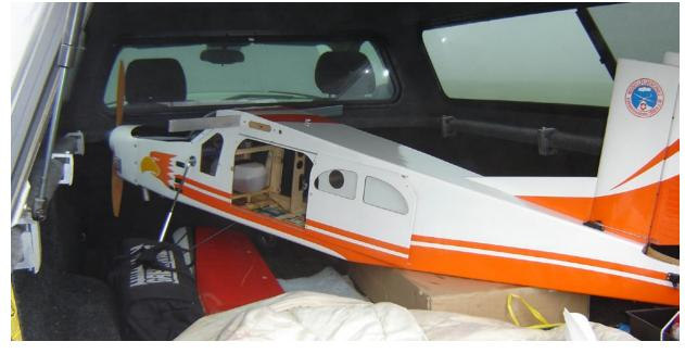
The 3+ meter span Pilatus tow tug has the side door open to reveal the 80 ounce fuel tank. The tow point is just visible at the trailing edge of the orange stripe on the top of the fuselage. The sliding side doors required additional fasteners in flight because they bulged outward into the airstream.
