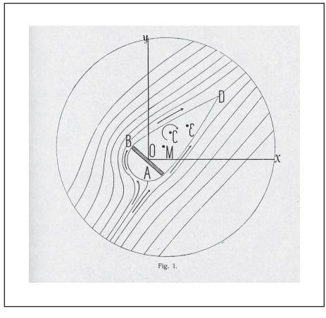
Figure 7: Nikolai Joukowski's diagram of the lift of a spinning vane device.
