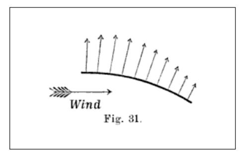
Figure 8: Lilienthal's 1889 diagram of centrifugal lift
