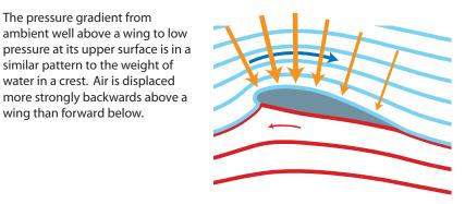
Earthquake (or Jell-O) wave crests and wing wave crests have similar internal patterns of motion. The sum of forces in a wing wave make the air above it act like it is under tension. Unlike solids in an earthquake or Jell-O wave, wing wave air is permanently displaced.
