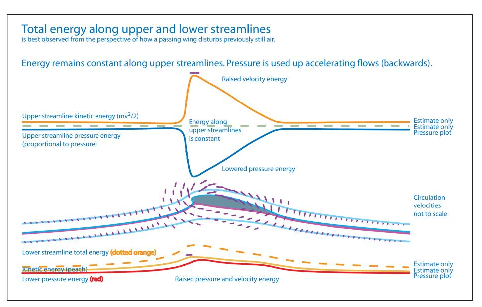
Figure 13: Total energy along upper streamlines is constant. Energy along lower streamlines is raised by a standing, raised pressure wave. Raised energy is carried along beneath the wing in the lower, pressure and momentum ridge wave. Along lower streamlines, pressure and velocity are simultaneously raised. This is typical of raised-pressure waves, which, like tsunamis, carry raised total energy. © 2011 Philip Randolph, 10° e393 streamline and CP plots by S. Allmaras
