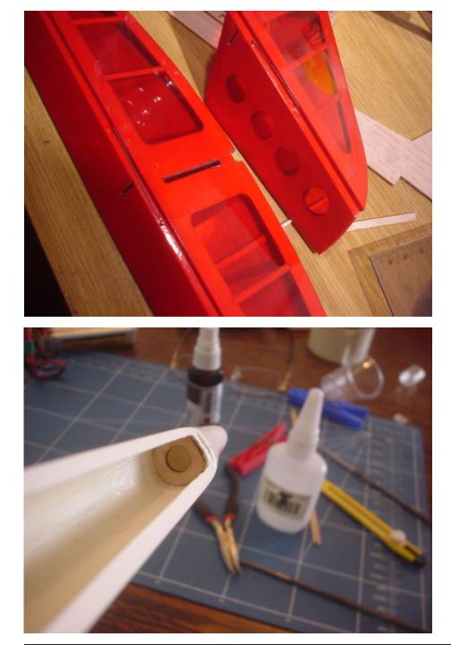
slide the tail group into the slots of the tail boom and add a few drops of thick CA.
