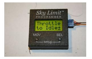
Setup with Throttle to Idle turned on
