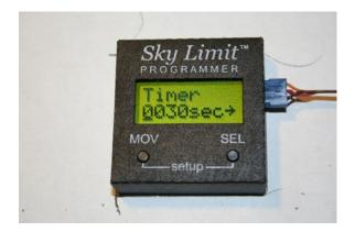
both together. For example, in an ALES contest you would set both, typically 200 M for altitude and 30 seconds of motor run time. For an F5J type contest you might only use the altitude limit. For some other LMR type events you might only use the time limit.
