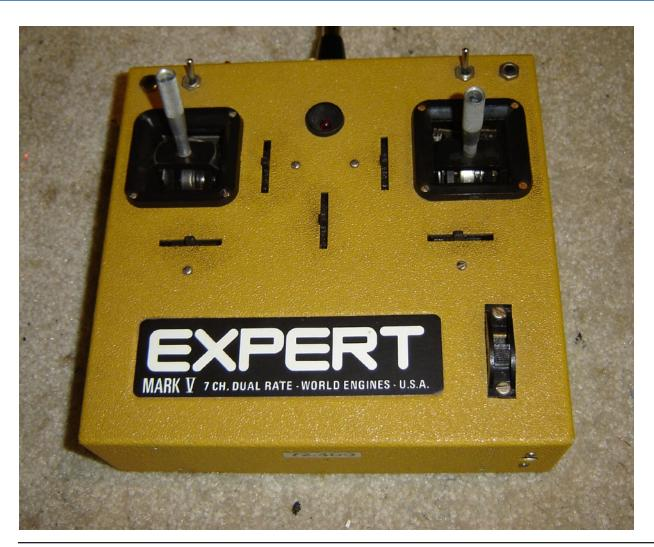
pulse widths. This is the old amplitude modulation scheme. Its main drawback is that, while the transmitter RF is switched off, the receiver in the aircraft is able to hear noise or interference which would drive the servos to one end or the other. This interference or "glitch" has sent many a model into an unscheduled landing sequence!
