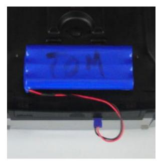
Photo 10: External battery connected.
