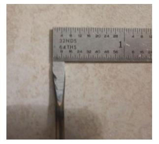
14. Now I needed a way to put the clevis back on. I flattened the other end to about 3/16".
