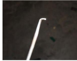
15. Bent it about 80 degrees. You can bend it up to 90, but the edge of my vise was a bit rounded. It actually turned out easier to remove, after installing the clevis, with less than a 90 degree bend.
