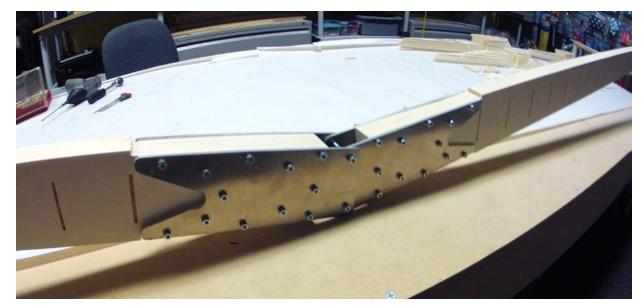
Main wing joiner assembly. Notice "fishplates" to prevent stress risers.
