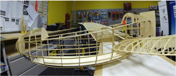
Fuselage under construction. Bottom photo shows the separated front portion with the joiner section being fitted. The result is a two-piece fuselage that bolts together on the field with a near invisible joint, as can be seen on the title page opposite.
