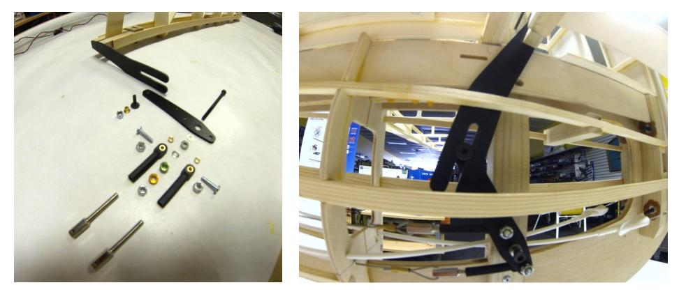
The various parts of the elevator control system. Two JR 8411 servos at the front of the rear fuselage section drive forked arms through a pull-pull cable system. The mechanism slides together as the stabilizer is mounted to the fuselage.
