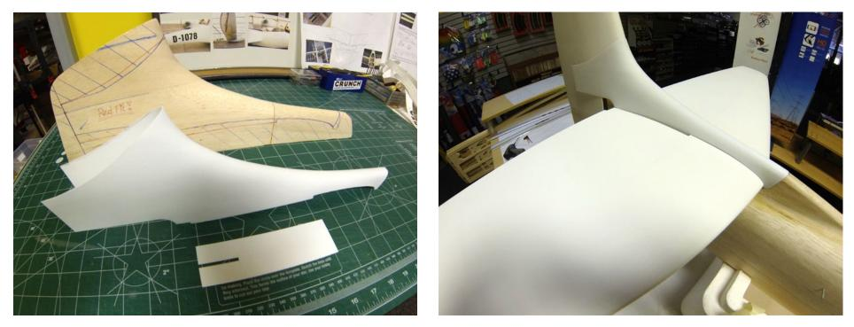
Left: The balsa master plug for the tail fairing sits behind the finished vacuum-formed finished product of 0.060" styrene. Right: The formed fairing in place, held by magnets at the front and fasteners on the vertical fin. The size of the fairing required a 12 inch by 24 inch sheet of plastic, so a new vacuum box had to be constructed to form the part.
