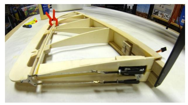
Internal elevator trim tab pull-pull cabling and servo.
