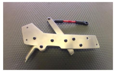
The custom-made tow release which is mounted below the nose of the Mg 19a.
