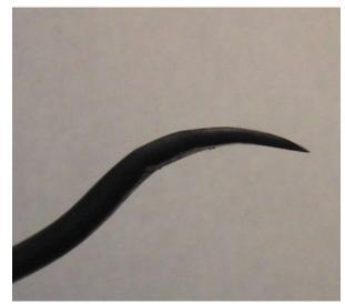
A final note: There's one last thing. Sharpen the end of the pry bar so it can more easily slide under the clevis.
