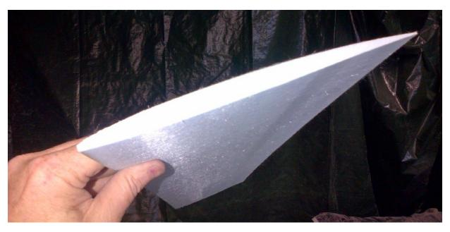
The wing core showing the thin section used.
