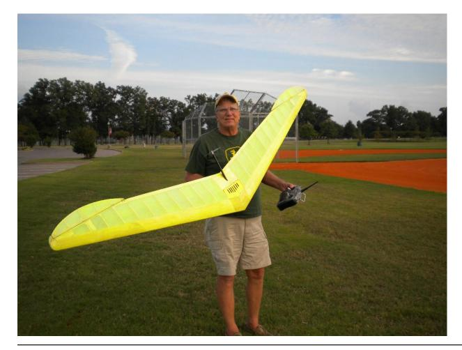
I thought I'd send a few photos of our latest 'wing, "Albatross." The Albatross weighs 2 lbs. 14 oz. and is powered by three cells with an MPi 2800kV motor direct drive.
