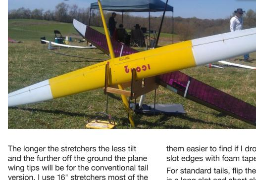
On the field, the Multi-Stand can be configured for either conventional tails or V-tails by turning around one side panel. The cant angle can be adjusted by making shorter and/or longer stretcher bars in the shop. Might be nice to have a couple of lengths made up ahead of time.
