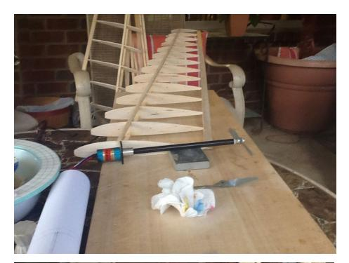
The extended drive is home-made. I used .125" music wire running in UHMW bushings and turned a chunk of 6061T-6 for the mount and prop driver. The shaft log is a piece of scrap tubing from a paraglider. MPi 2800kV motor turns a 7X4 direct drive at 21K and if Albatross hangs, we will put roller bearings in the shaft log when the bushings wear out, but this was a budget build with parts that we had or could make.
