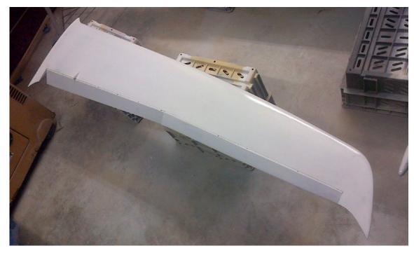
Glass the concave hinge areas with 49g/m<sup>2</sup> cloth. This helps as a sub spar and anchors the hinge pins. Give it a light sanding when cured.
