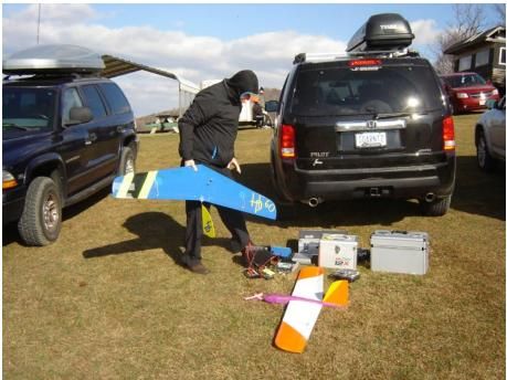
This slope ship was equipped with wingeron steering. Servos in the fuselage controlled each wing panel. The panels rotated around the massive steel wing rod. Here the pilot tries to free the bent rod which had partially jammed the steering.
