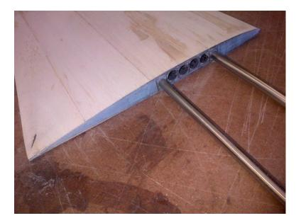
▲ Joiners in place, ballast tubes open
