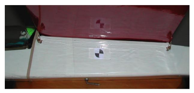
This Sophisticated Lady was made 5 ounces lighter by using a pair of CGAs. The natural CG of this plane without CGAs is 1.5 inch aft.
