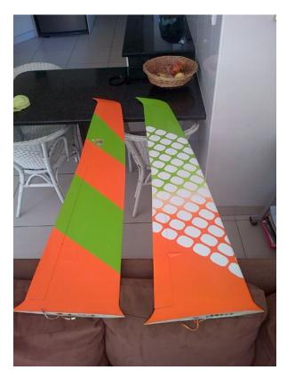
Bottom and top surfaces after application of 2-part automotive paint
