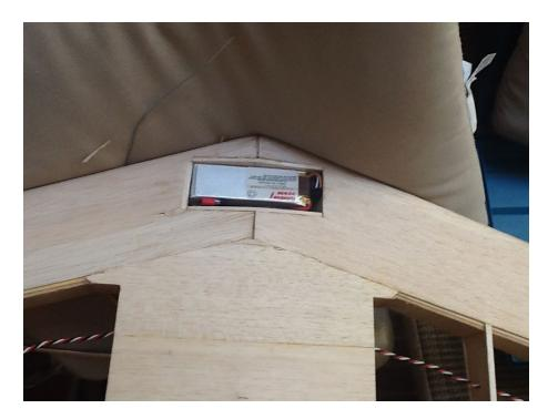
Above: Battery box on the lower skin.. 2100mah... Overkill but we had the batteries on hand and it needed the weight.
