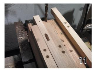
Mark for slot. 3/4" to 1" wide. This helps keep the screw from jamming when at different angles during clamping. See Photo 9.
