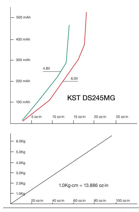
We tested the DS245MG with 4.8V and 6.0V. The accompanying charts show the torque and current as related to the position signal being received by the servo amplifier, 1000µsec-2000µsec, 1500µsec neutral.
