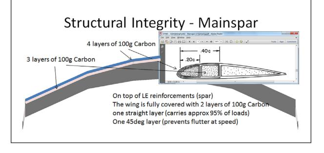
suffer at these locations, and also this provides maximum stiffness to the parts that need to be held in place in the height of the wing end - mainspar, alignment dowel, hole for wires to the servo in the outer panel. I even considered placing plywood ribs in the joining place between the cores that would bond together, but finally reverted from this. I do not feel that it is needed.
