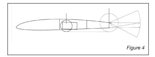
are drooped to provide additional lift or are raised to provide additional drag in crow mode. The circles are still used to define the pushrod attachment points, however different size circles will be required to reduce the angular deflections from the 90 degree total rotation of the servo to the deflection desired for the aileron.
