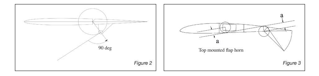
line with radius equal to the distance from the hinge to the pushrod connection. Then draw another circle around the servo shaft equal to the length of the servo arm and draw a line tangent to the circles. Where the line touches the circles is the correct locations of the pushrod connections to the servo arm and control horn.
