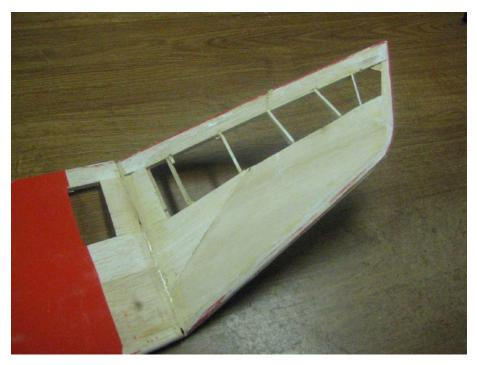
Photo 9: Left wing tip repair.
