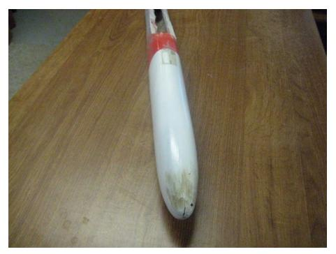
Photo 7: Nose cone damage.
