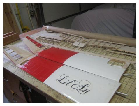
Photo 10: Wing repaired complete, waiting for recovering.
