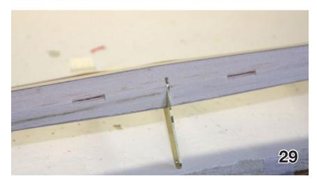
to let the hinges go into the elevator a bit further, thus reducing the hinge gap when the elevator is hinged. I set it up for around 1/32" gap. See pix 28 - 29.
