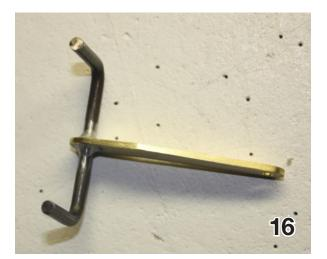
The elevator leading edge piece must also by notched to allow the control horn assembly to fit flush with the aft surface of the leading edge. I used a razor blade, X-Acto, and small file to do this. It might have been easier to make this notch before I glued on all the elevator ribs! Check the fit of the control horn assembly and block and glue into place with 15 minute epoxy. See pix 17-21.
