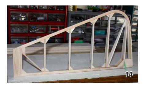
Draw a centerline on the LE, mark the locations of the hinge slots, and cut the slots.
