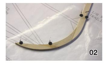
into the slot in the end of R1 to match the trailing edge piece. Glue R1 to the leading edge and trailing edge. See pix 6 and 7.
