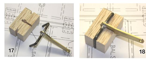
19. Notching elevator leading edge for control horn assembly. ribs; make sure the trailing edge is held flat to the building surface with pins or whatever when you glue in the webs.
