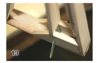
10. The 1/16" thick G-10 rudder horn cut and sanded to shape.
