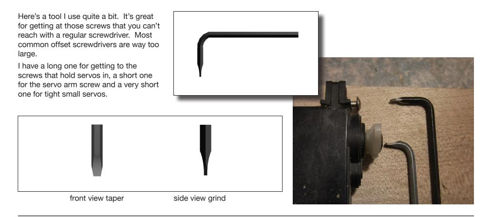
This tool saves taking the servo out, when all I need to do is move the arm a notch or two.
