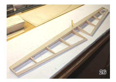
ply piece using CA+ on the center block and ribs, and CA on the webs. Add the 3/16" wide, 1/32" ply cap strips to the ribs with CA. Sand the ends of all the ply pieces flush at the elevator tips. See pix 26 - 27.
