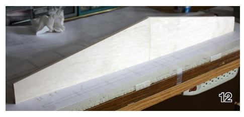
This completes the basic construction of the horizontal stab. The elevator is next.
