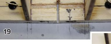
After the elevator control horn assembly glue has cured, sight along the ends of the ribs and adjust any if required.
