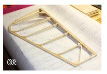
07 & 08. Rib R1 installed; angle braces installed; 1/4" and 1/8" gussets installed
