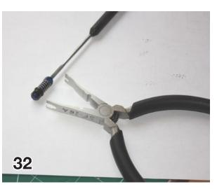
to fit around the sleeve on the Sullivan connector. You simply squeeze the pliers to compress the connector sleeve and release it from the ball. This makes it quick and easy to use inside a fuselage. See pix 32 - 33.
