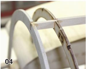
If you have a vario and plan to use a total energy (TE) probe, now is the time to install the TE tubing.
