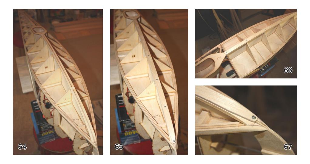
Mark the skid where the holes will be drilled. There should be one screw at each of the three blocks on the keel, one screw between each block, and one screw at the nose for a total of seven holes. Tape or clamp the skid in place, making sure it is centered, then drill the seven holes with a 1/16" drill bit to a depth of about 5/8 inch.
