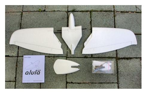
Alula-Trek kit contents: five molded foam parts - wing halves with elevons pre-hinged, fuselage with hatch, vertical fin. Also a complete hardware bag and the superb construction, trimming, and flying manual.
