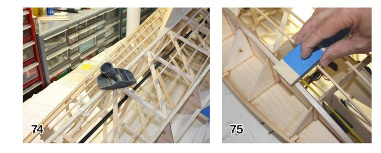
I lived dangerously and planed mine close, finishing with a sanding block, first with 100, then 220 grit.
