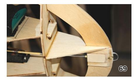
On the screw holes in the basswood blocks, I hardened the threads by applying CA into the screw holes after removing the screws.
