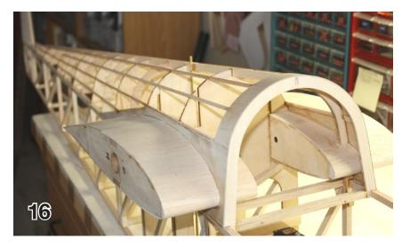
I like to start with the stringers that are glued to the edge of the 1/32" ply center section fairing pieces. Use a straightedge and sight along the stringers from the end to make sure they are straight.
