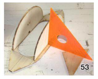
If you haven't already done so, notch out the balsa cross piece at the bottom of fuse former F6 to match the notch in F6. Fit check the wheel well, make any adjustments, and glue to the keel, bottom stringer, and F6 with CA+. See pix 55 & 56.
