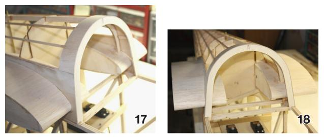
The area over formers F4 and F5 is covered with 1/32" ply. Make a paper template from manilla folder or similar material, and cut the 1/32" ply a bit oversize, then fit it to the formers. Once you have a good fit, add some 1/4" wide ply tabs on each end on the inside - these will reinforce the glue joints at the ends. Glue the ply on and sand the front edge flush with F4. See pix 16 - 18.
