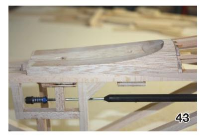
40 - 43. Using a Monokote separator, a micture of epoxy and microballoons is used to get the stabilzer mount to exactly fit the stabilizer.
