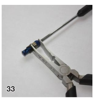
32 & 33. Modified helicopter ball link pliers are used to retract the sleeve and release the ball.
