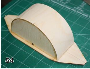
53 - 56. Construction of the wheel well. Make sure to apply three coats of Poly-U to the inside of the well to seal it from dirt and moisture.
