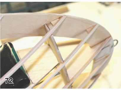
Use the plan templates to cut the 1/2" balsa contour blocks, and the 1/8" thick X 1/8" wide ply pieces that go underneath the contour blocks (to reinforce the thin edge after sanding).
