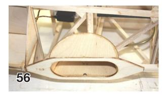
Add the F6A formers to both sides of the wheel well, paying attention to where they are positioned relative to the holes through the WW sides.
