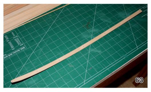
61 & 62. Three layers of 1/32" plywood laminated with 15 minute epoxy and clamped to keel for shaping. Note regular clamp at nose.63. Finished skid.
