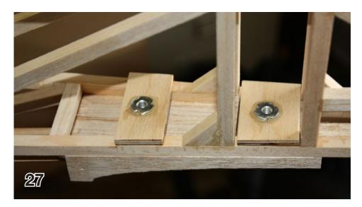
I taped a piece of brass tube onto my drill bit for an extension to drill the 1/4 holes.
