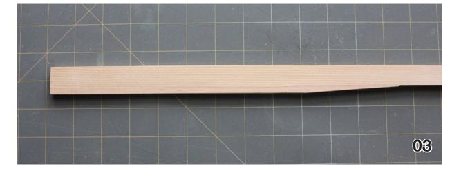
01. Splice joint; 12:1, so splice is 9" long.
