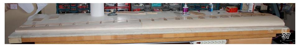
Before gluing the top D-tube sheeting, the entire wing needs to be pinned down.
