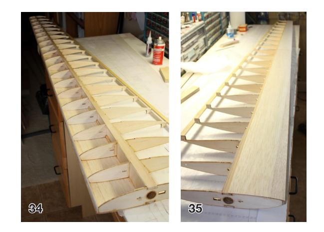
D-tube sheeting to fit. The inboard piece will need some additional 3/32" sheet added to make it wide enough. Leave 1/8" extra on the root end, leading edge, and tip end.
