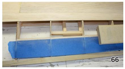
65. The first three webs are glued into place on the wing side of the aileron bay.
