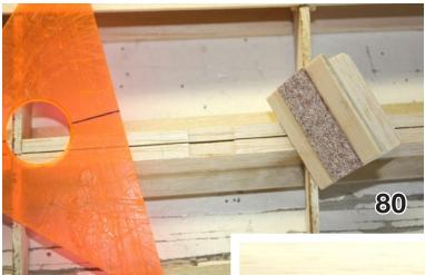
has a center line marked on it – I hold the triangle down over the hinge line with one hand and operate the sanding tool with the other hand.
