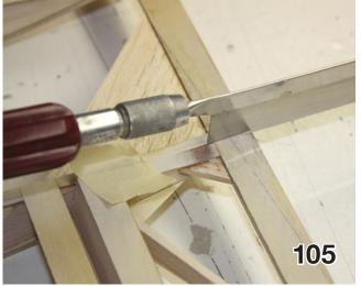
Use a razor saw to cut through the remainder of each rib from the bottom side. See pic 104.
