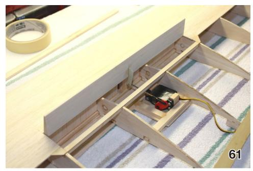
59 - 61. The spoiler pushrod runs under the upper spar cap. The servo arm must have enough travel to push the spoiler fully open.
