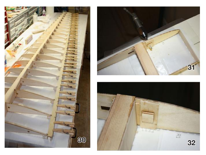
30. This photo shows the entire trailing edge glued up and being held in place with pins and clamps.
