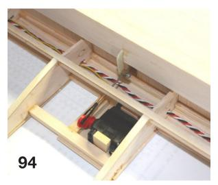
Route the servo wires between the two servos and the Molex connector at rib 1. See pic 91.
