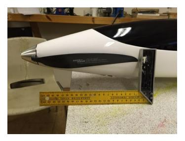
Left: The first kits were supplied with a Aeronaut Cam prop that isn't up to the RPM's and were replaced by Staufenbiel's own product. Middle: Shown here besides a 22x10 propeller. Above: Impressive size for an electric motor when you are used to the 13" and 14" sizes.
