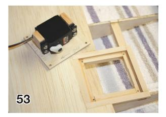
Cut and fit 3/32" plywood doors for the spoiler and aileron servo mounting frames.
