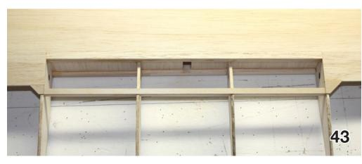
Cut and fit the small 1/32" ply gussets, and the strip of 1/32" ply that goes on top of the 1/4" square basswood, and CA into place. See pix 42 - 44.
