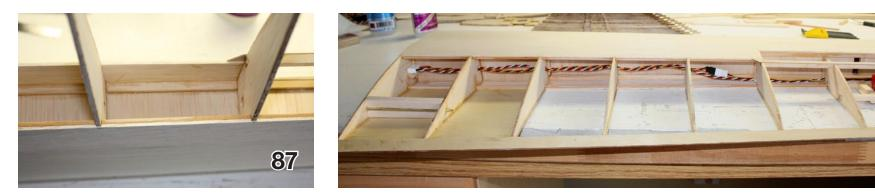
I had originally intended that the aft edge of the wing sheeting remain unsupported. However, as I handled the wing panel it became apparent that the unsupported edge would eventually get cracked due to handling loads. Therefore I have added pieces of 1/8" square basswood between the ribs all along the aft edge of the top and bottom sheeting. See pic 87.
