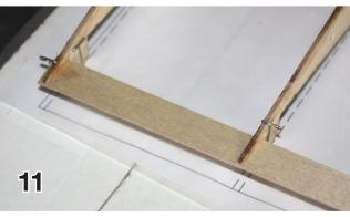
Glue R3B to the outboard side of rib 3, centered on the wing socket tube hole. R3B serves as the wing tube stop when inserting the wing tube later on. See pic 10.
