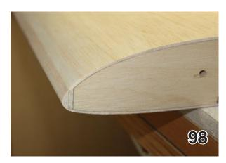
Use a razor plane and sanding blocks to shape the leading edge, checking often with the sanding templates as you progress. See pix 97-98.
