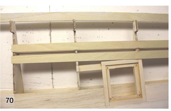
Cut the two aileron end ribs to fit between the rear webbing and the wing trailing edge near ribs 12 and 21, and glue into place - these should be positioned with a 1/32" gap from the wing ribs. Add the 1/8" balsa gussets. See pix 71 and 72.
