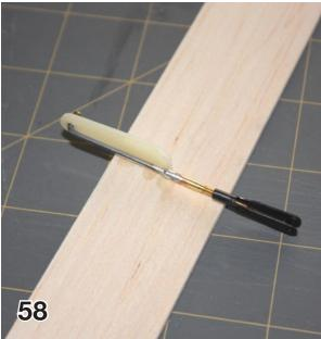
I still use the Kwik Link to connect to the servo arm, but at the spoiler horn I am now using a Great Planes Screw-Lock connector.
