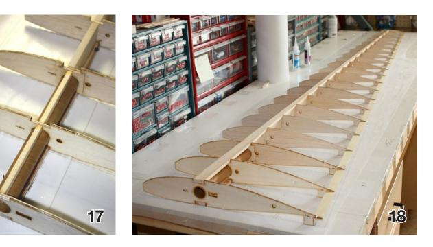
Fit check the upper spar cap again and sand the top of any webs if needed.
