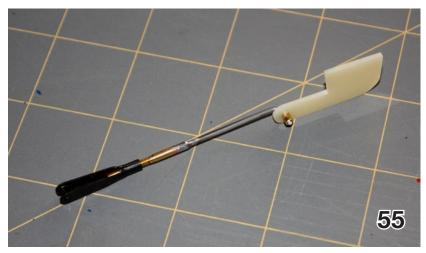
Copy the spoiler and aileron horn shapes off the plan and glue the templates to the G-10 with rubber cement. Cut the horns out a bit oversize and sand to final shape.
