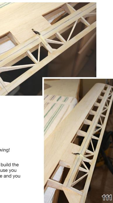
109. Hinge dry fit showing relief in wing and aileron for the center of the hinge.
