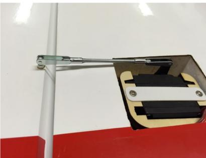
The wing comes in four parts, divided at the aileron/flaps and flaps/ fuselage. The flaps could have a nice career as barn doors!
