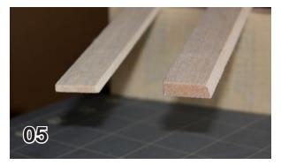
At the line closest to the end of the spar cap make two marks 3/8 inch apart centered on the spar cap. At the next line make two marks 1/2 inch apart, and at the next make two marks 5/8 inch apart.
