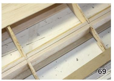
67. Aft (aileron face) webs being glued into place. machinist ruller used to get 1/64" spacing from front webs.
