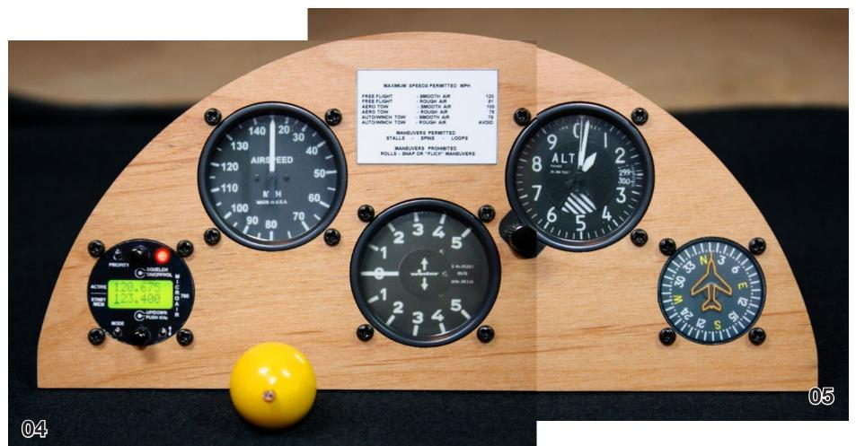
04 and 05: Composite image of the completed instrument panel. Instruments, left to right are Microair radio, airspeed indicator, variometer, altimeter, and compass. The large yellow knob at the lower left is, of course, the tow release. The placard provides maximum speeds permitted in mph, plus maneuvers permitted (stalls, spins and loops) and maneuvers prohibited (rolls and snap or "flick" maneuvers).
