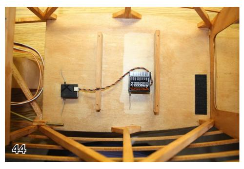
The wiring harnesses coming from the wing roots need to be tied down with two tie-wraps which use the holes provided in former F6. See pic 43.
