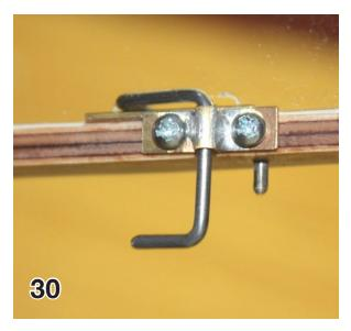
30 - 32: The latches are mounted on the canopy side rail with cut off #2 sheet metal screws. These photos show the right side latch in the open position.
