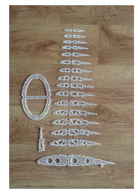
The printing time is quite high, around 30 minutes for a 29 cm rib, but this is mainly because the printer nozzle diameter is 0.35mm, which is good for detailed objects but not necessary for this particular job. The nozzle could be changed and that would reduce the printing time in half.
