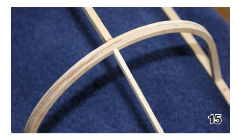
Again using the taped sanding block, bevel the aft half of C2, bevel C3, and bevel C1.
