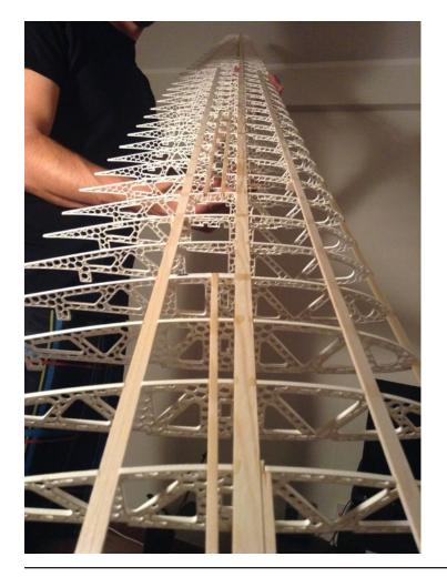
Being the owner of a 3-D printer for quite a while, I have been doing a lot of small things like servo trays, dummy engines, pilot heads (photo below), bits and pieces. But this time I decided to use the printer on a large scale, so I've been printing ribs and frames for the Jilles Smits' 4.7m KA6E (photo at left).
