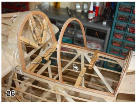
What you want is a template that fits as closely as possible so later you can glue the plastic onto the frame with the frame clamped into place on the fuselage.
