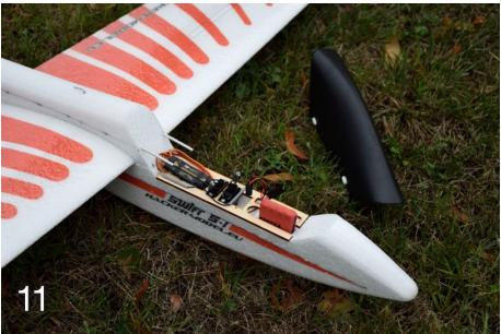
A plywood tray receives the 9 to 12 gr servos — Tower Pro MG90 Servo 9g metal in my case. The receiver is located behind the servos and should be small size (Photo 11).
