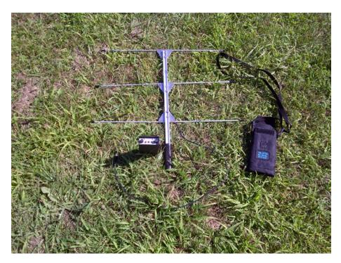
Walston receiver, antenna and carry case. The carry case frees one hand to hold the antenna.
