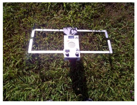
The CSI receiver and antenna are shown assembled together and ready for use.
