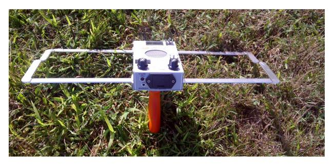
The CSI receiver and antenna are shown assembled together and ready for use.
