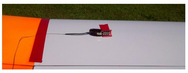
This Walston transmitter, roughly  $1/2 \times 2$  inches, has Velcro glued around its encapsulated end and allows easy removal when replacing batteries. The red electrical tape is to hold the batteries in after losing the plastic tube.
