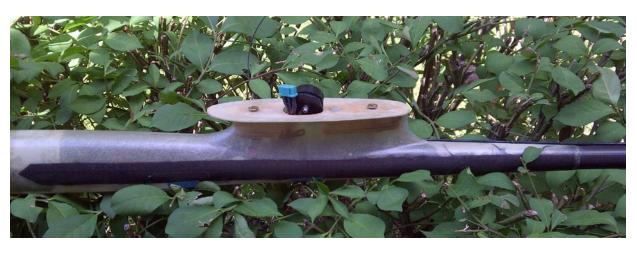
The CSI PR-1B transmitter slides right into this Supra's fuselage where the ballast tube should be. Its antenna exits at 90 degrees to the fuselage, above and away from the carbon strips.
