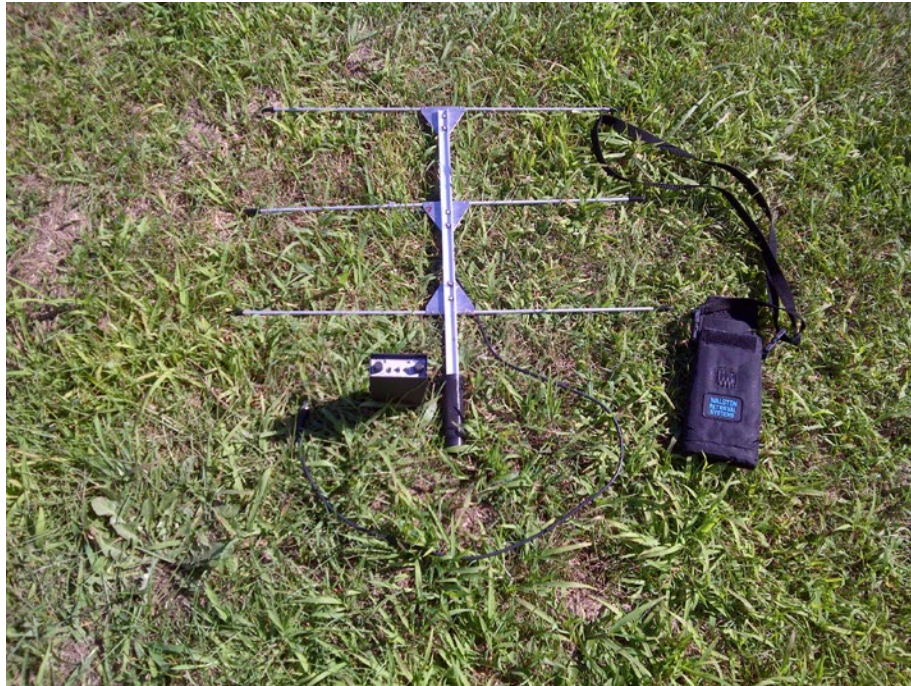
Walston receiver, antenna and carry case. The carry case frees one hand to hold the antenna.
