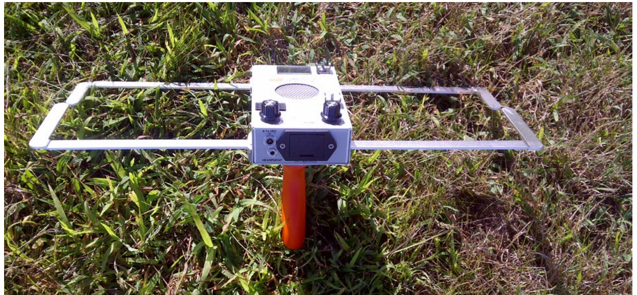
The CSI receiver and antenna are shown assembled together and ready for use.
