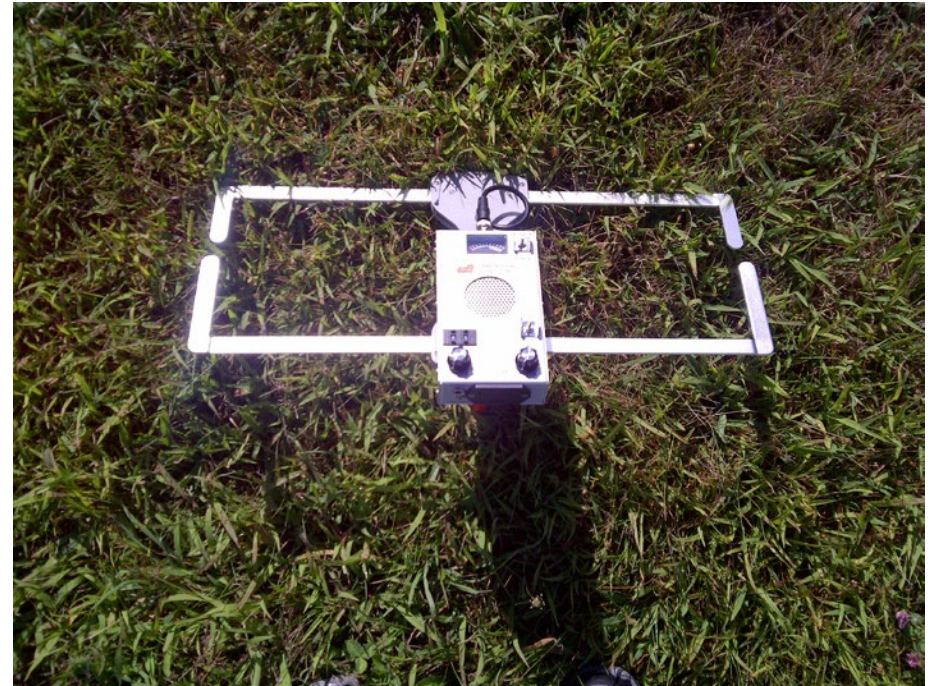
The CSI receiver and antenna are shown assembled together and ready for use.
