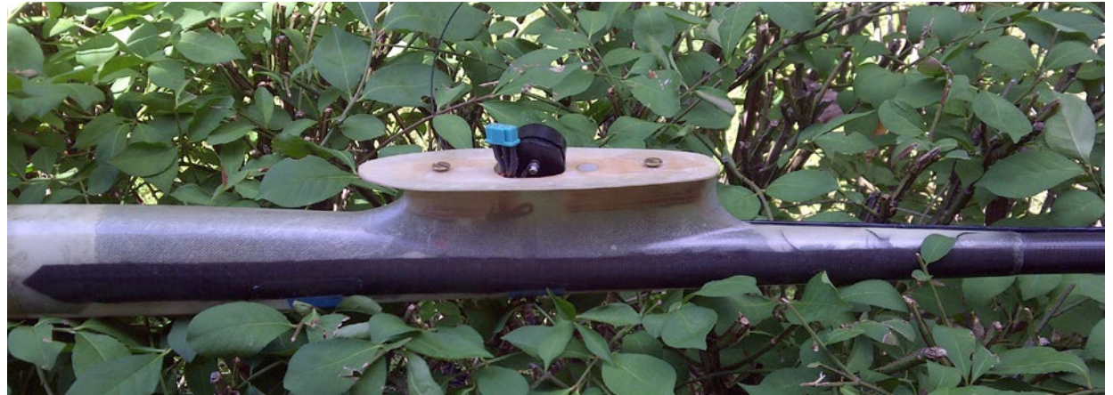
The CSI PR-1B transmitter slides right into this Supra's fuselage where the ballast tube should be. Its antenna exits at 90 degrees to the fuselage, above and away from the carbon strips.
