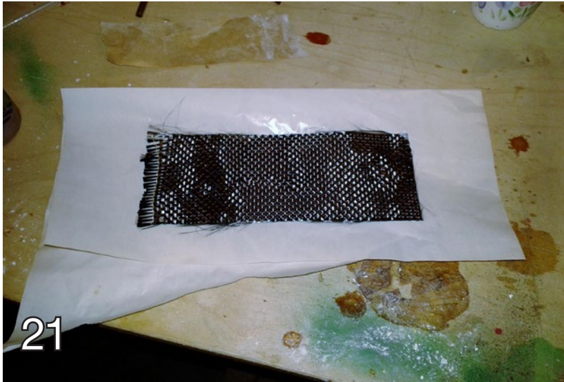
21. Cut and wet out a piece of carbon cloth.
