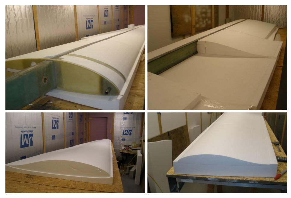
Upper: Left wing core showing root face, alignment pin and spar assembly. Above: Wing core showing the airfoil shape.
