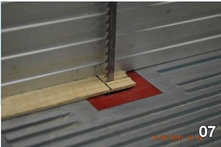
tapers from 3/8" high at the root to 1/4" high at the tip. The spar caps are 15 inch long, 3/8" wide, and trimmed to length after assembly.
