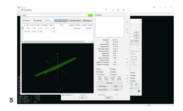
Each flight mode is set up as a different plane. I recommend doing this so you can compare polars across flight modes.
