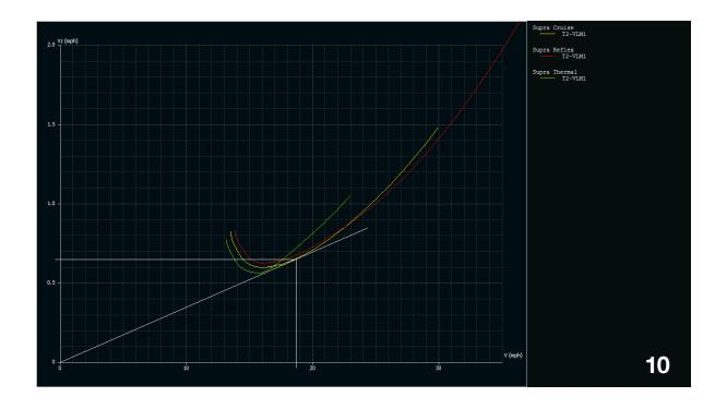
XFLR5 is an incredibly powerful program and with this simple introduction to it you should be able to explore many more options, like changing the airfoils, aspect ratios, or tail moments. The bottom of the thermal mode curve is nice and flat, giving you a speed range from 14.5 to 16.5 mph with little penalty for deviating from the optimum at 15.5 mph. This is one of the reasons why the Supra is so easy to fly.
