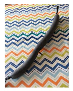
Here is a new tool I made to hold a patch inside a fuselage or similar repairs. Made from a bicycle tire tube.
