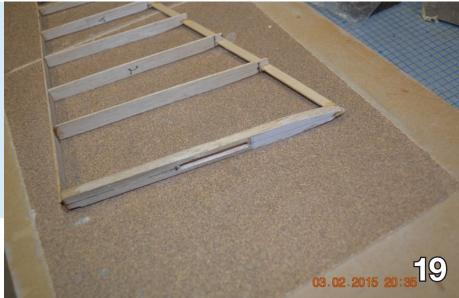
The root rib blank is 1/4" thick soft balsa and slotted for the stab horn. A template for a symmetric leading edge is glued to the root rib ahead of the stab horn. Draw lines at the rib locations on the inside of a fin skin.
