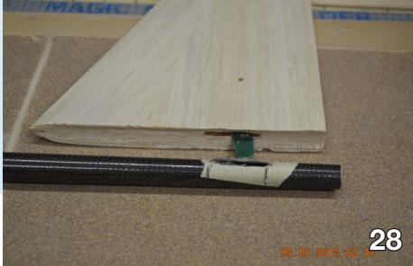
Hold the assembled rudder against the fin and trace the fin on the rudder leading edge. Trim the leading edge and ribs oversize before sanding the rudder to near final shape.
