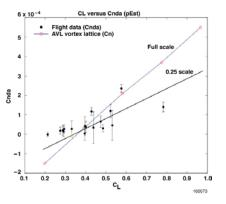
Figure 6. Yawing moment due to aileron deflection coefficient versus lift coefficient.
