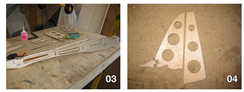
Photos 1, 2, 3: Basic fuselage construction Photo 4: Vertical fin and rudder
