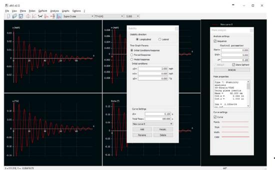
The decreasing amplitude shows that the plane will recover from a perturbation and return to level, stable flight hands off. Progressively moving the CG back will reduce the time to recover to stable flight, as shiown in Screen 17.
