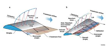
Figure 2. Prandtl's elliptical and bell spanloads explained.
