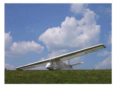
the aircraft lifts off. After take-off the pilot retracts his legs and puts them on rudder pedals. A sliding slat-type construction behind the pilot's back can be released in flight to provide a seat.
