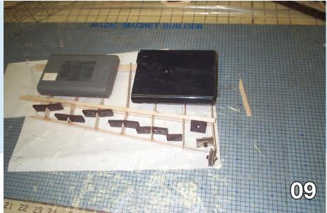
The leading and trailing edge rib blanks are then glued in place. I have found that thick CA works best for attaching the rib blanks to the spar. After all rib blanks have been installed, slide the leading and trailing edge in place and glue with CA (Photo 9). Install a 3/8 inch wide 1/16 balsa tip between the leading edge at the tip rib and the trailing edge 2 inches from the tip rib. Glue the spar caps to the tip and trim flush with the tip.
