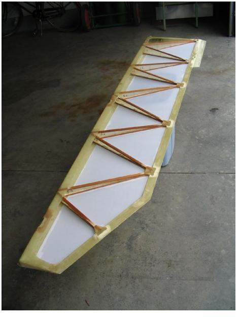
Above left: Interior details of the wing showing the aileron control system. Left: Open spoiler. Note the composite rib structure. Above: Elevator under construction.
