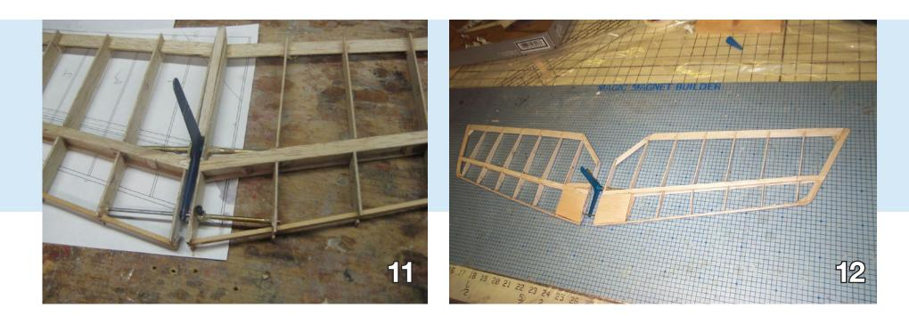
When satisfied with the alignment, epoxy the other stab pivot wire tube and the forward stab wire in place.
