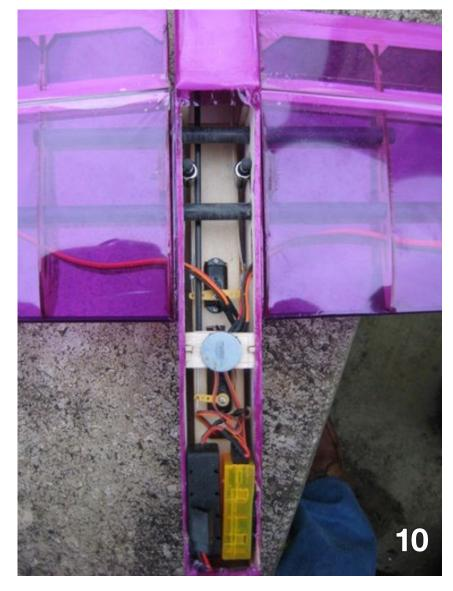
Photo 8: Component parts assembled Photo 9: Servos mounted in fuselage Photo 10: Internal view of the fuselage with wings attached
