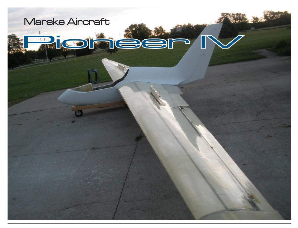
The Marske Aircraft 15 meter Pioneer IV has made a few low hops so far off the winch before winter stopped operations. It shares essentially the same planform as the Pioneer III, with only a minor change to the trailing edge contour in the area around the outer end of the central elevator. Huge differences appear in the airfoil used and the construction materials.
