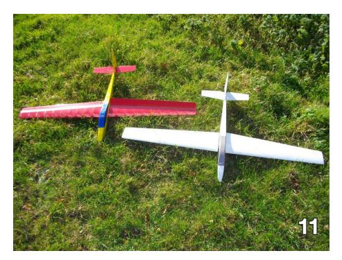
Photo 11: (L) Aileron version, (R) pivot wing version
