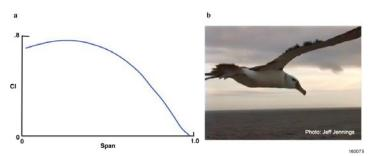
Figure 10. The local lift coefficient (Cl) and the beginning of stall on the wing of a wandering albatross.
