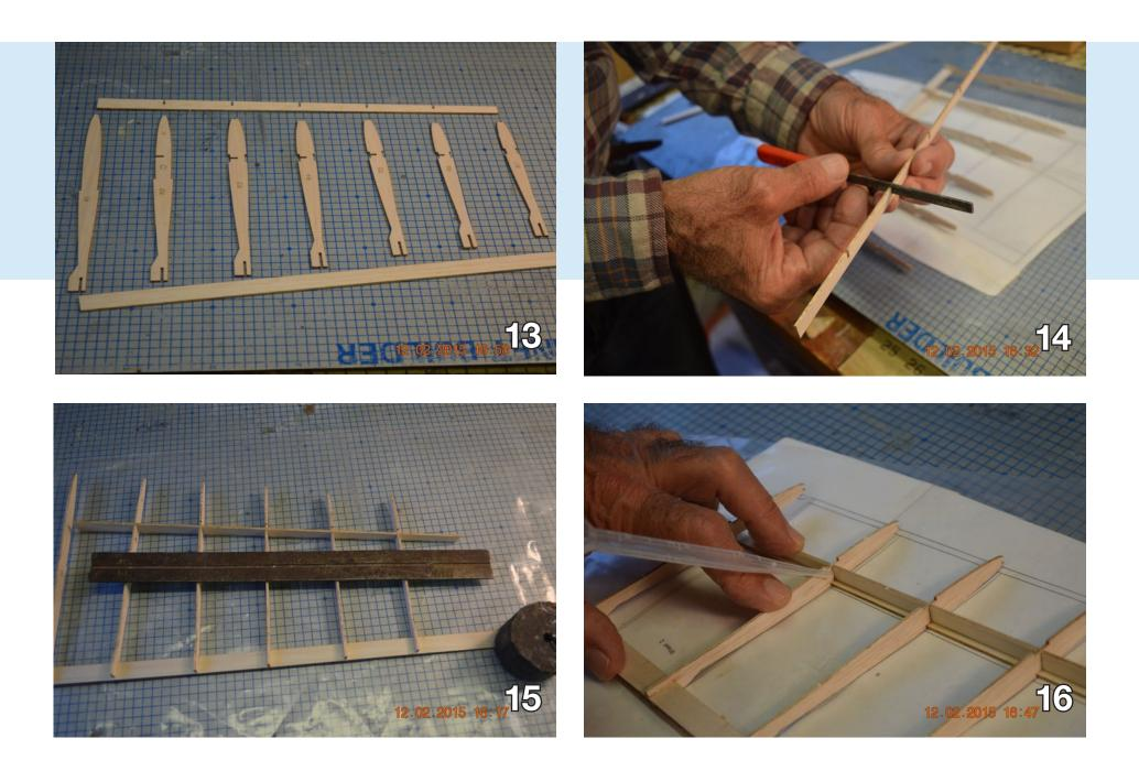
The egg-crated rib and spar can be aligned with the desired sweep before gluing with CA.
