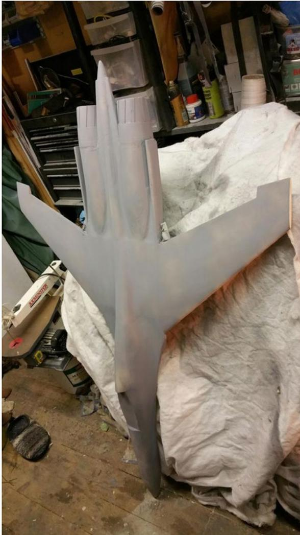
27. I braved the cold this evening and cracked on with a first guide coat of primer on the Flanker. The fins, sub fins, ailerons and elevators are now drying out with their first layer of glass too. All coming along!
