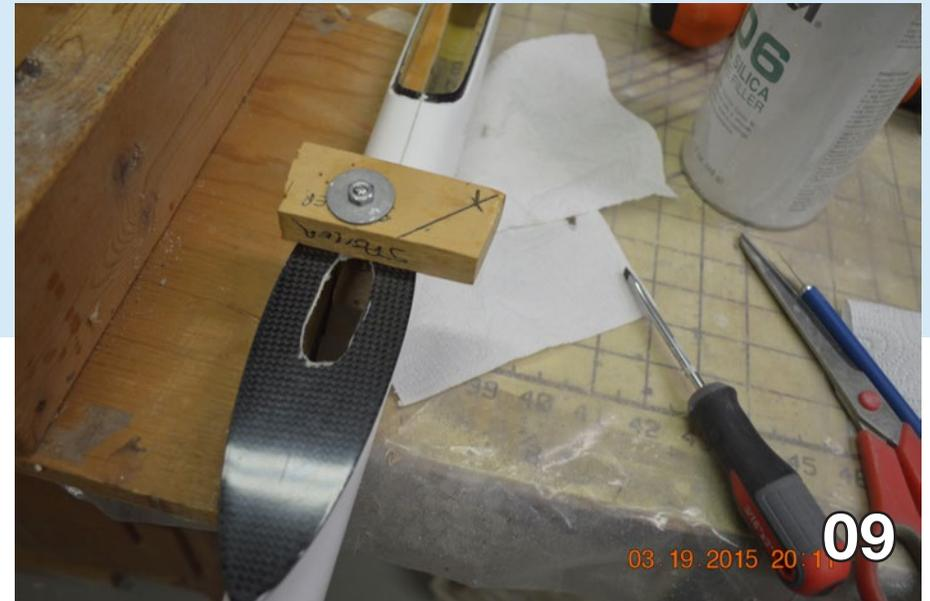
the location of the bolt and drill a hole for the T-nut just aft of the mark.
