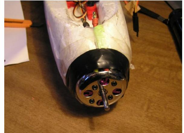
9: Martini cap and motor installed in EasyGlider Electric.
