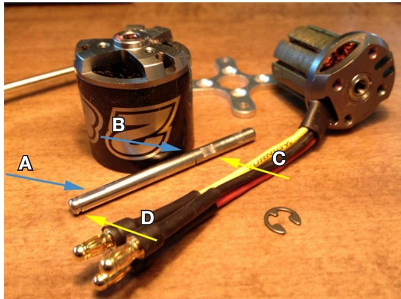
1. The 2836 1800kv outrunner disassembled. The shaft shows the old (A) and new (C) machined flat spot and the old (B) and new (D) machined groove for the e-clip.
