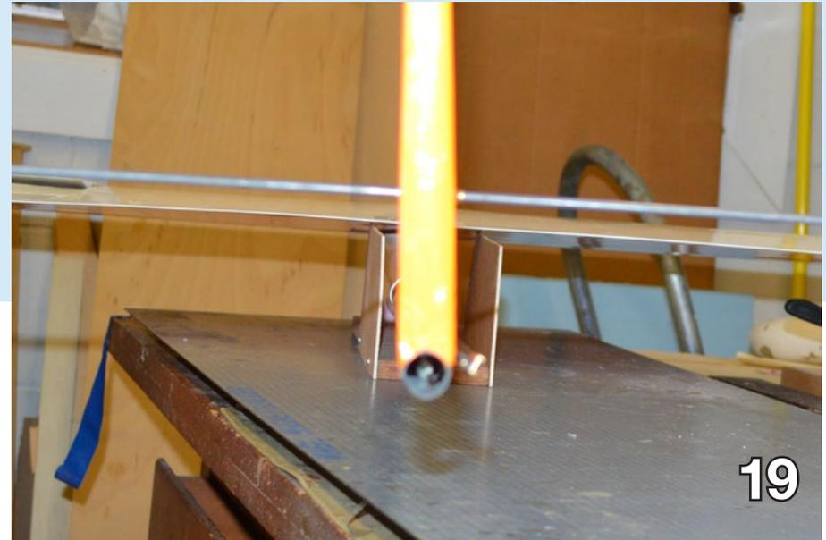
adjust the tilt, enlarge the stab bearing hole in one side of the fin.
