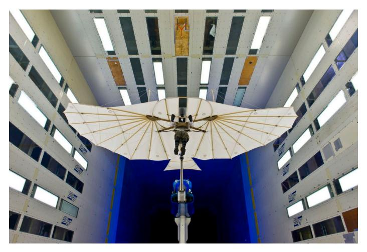
Flow test in the wind tunnel
