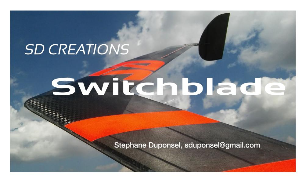
The SD Creations Switchblade is a 1.2m wing span ARTF (almost ready to fly) discus launchable flying wing. It comes with servos and the battery already installed. All you need to do is add your receiver.
