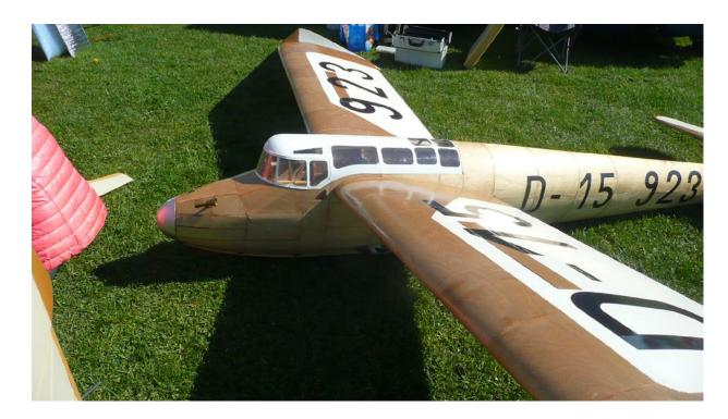
Two photos of the half scale two-place Minimoa Mo2a. This model had a wing span of over 7 meters, was built entirely of wood, and was extremely detailed.
