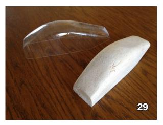
Photo 27: Everything is painfully sanded to the final shape, making sure of its symmetry and that it fits nicely on the fuselage.
