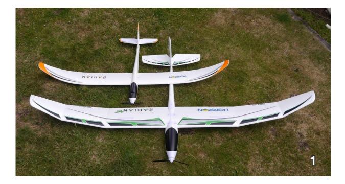
the plane is, overall, just about a 30% scale-up of the Radian 2m. Tail surfaces are noticeably larger.
