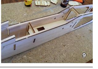
Photos 1 - 5: The fuselage sides are cut in 2mm balsa, and 5x5mm balsa strips are glued all around the edges. (See plan.)
