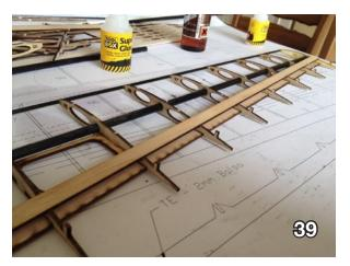
Photos 38 - 39: At this stage, the wing is rigid enough to be removed from the bench, turned over, and the top balsa strip is then glued in place.
