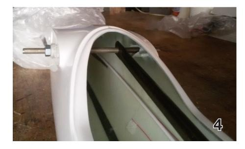
5. With the alignment tube still in place, a disk sander can be used to carefully set the fuselage nose edge contour to the thrust angles which have now been built in.
