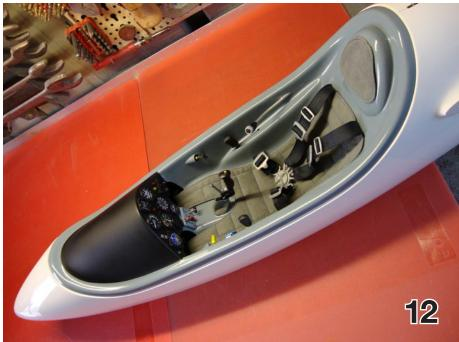
and tow release servos allows a custom cockpit to be fitted.12. All equipment is hidden below the cockpit interior.
