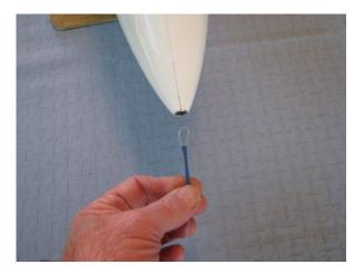
1. Heat shrink slid forward to make a small loop - easy to slide into the tube.
