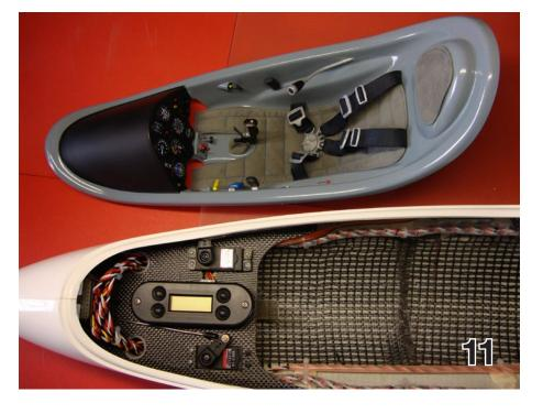
9. A double 2600 mAh Lipo battery was configured to fit in the nose (note the cells are offset).
