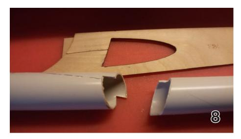
8 and 9. A plywood template was used on a PVC tube to achieve the proper contour for the exhaust opening. The left piece in Photo 8 shows the penciled outline as well as the notches which allow the forward portion of the outlet to be inset in the fuselage. The finished outlet is shown in Photo 9.
