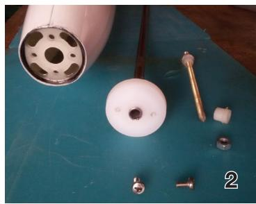
2. In order to get the thrust line set up properly, a simple alignment tool is constructed. Precut the nose so it's 1 - 2 mm longer than the final size. A PVC pattern is then forced into the fuselage. It will hold the motor frame in place while the epoxy cures. Note the tube extending back from the center of the PVC pattern. See also Photo 4.
