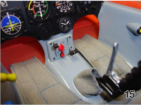
13 - 15. These photos show the cockpit details of Gino's Tangent Modelltechnik ASH 26. Gino assembled some of the cockpit interior with readily available retail parts, like the instruments and the microphone, but most of the pieces were made or assembled from small parts - pins, LEDs, etc. The seat upholstery was sewn by Gino's wife.
