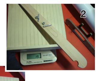
1. Gino innovated when it came to placing the elevator servo in his Tangent Modelltechnik ASH 26, moving it from the cockpit area to the vertical fin. This allowed a direct elevator drive. Here you see the various parts used in this modification.
