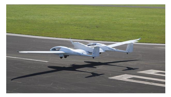
propel the aircraft. A high-performance lithium battery covers peak power loads during take-off and when climbing. If the hydrogen required for the fuel cell is generated via electrolysis using power from renewable energy sources, the HY4 can fly without generating any emissions at all. The aircraft is operated by the DLR spin-off H2FLY.
