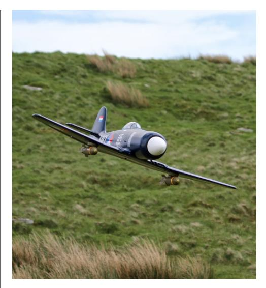
Phil Cooke's PSS Hawker Fury seen flying fast and low into the bomb release zone at the recent PSSA Fly-In at the Bwlch, South Wales, UK. Model spans 60" and has an AUW of 8lb – all black EPP construction with brown paper and PVA covering. Finished in a Dutch Navy scheme. Bomb release system by HobbyKing worked well! Photo by Andy Meade – PSSA – more info at <http://www.pssaonline.co.uk
