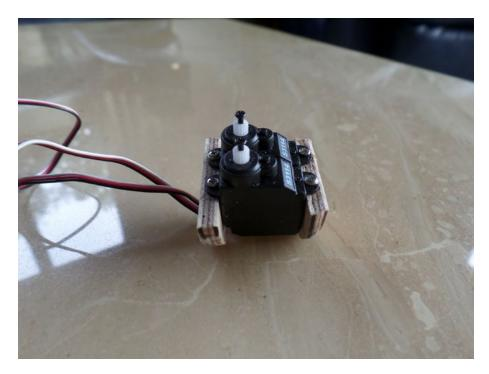
Rudder and elevator servos mounted to bulkhead to be glued into fuselage
