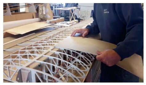
3 - Fixing the plywood to the top of the wing
