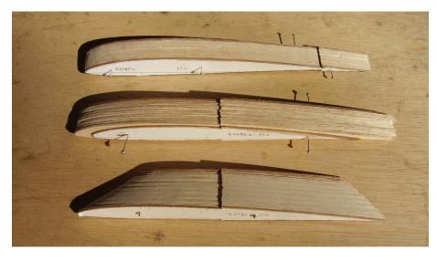
Figure W3: Wing rib stacks between master ribs
