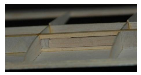
Figure W13: Tip joiner spacer wedge installed
