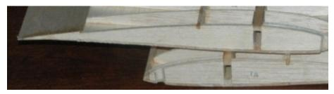
Figure W14: Wing mounting bolt notches at the front of the root ribs
