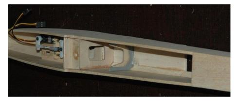
Figure F5: Mid-fuselage bulkhead installation
