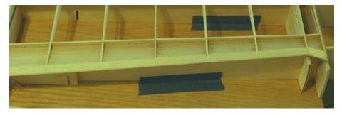
Figure W7: Trailing edge construction
