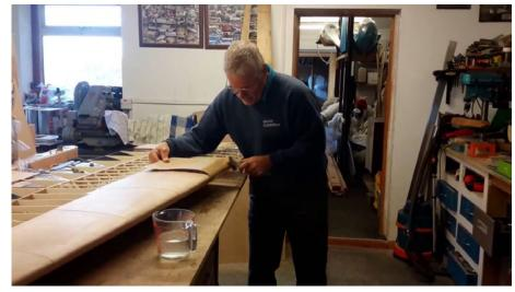
5 - Bending the panel around the Leading Edge and fixing the sheet to the underside
