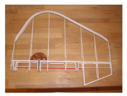
Rudder with the drive element in construction
