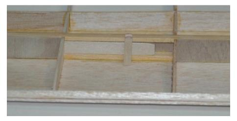
Figure W12: Tip Joiner in the wing spar with the spacer wedge in front
