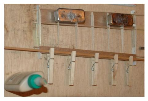
Figure T5: Closing the stab trailing edge
