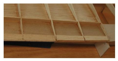
Figure W8: Trailing edge reinforcement — wedges on the left are shaped, on the right are as installed
