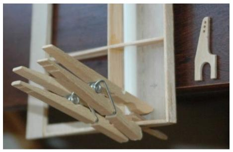
Figure T3: Control horn installation
