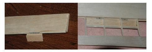
Figure W19: Spoiler installation details
