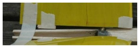
Figure F11: Tail spacers taped to the tail panels
