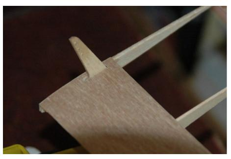
Figure T4: installed control horn
