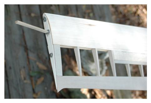
Figure W16: Assembling the tip joiner, first tip rib and guide pins
