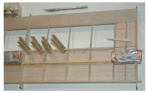
Figure W10: Installing shear webs at the back of the D-box
