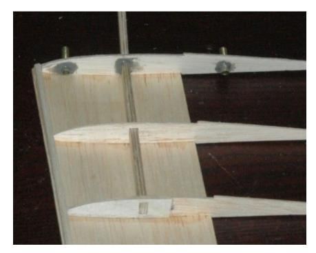
Figure W22: Installing the spar joiner and first three ribs
