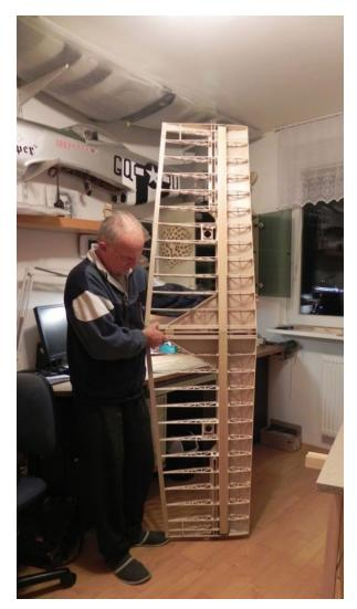
Middle part of the wing is already free from its assembly preparation, and the lower part still needs to be covered
