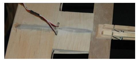
Figure F7: Rear wing mount clamped with clothes pins
