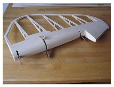
Rudder with skin made of balsa, pivots and drive
