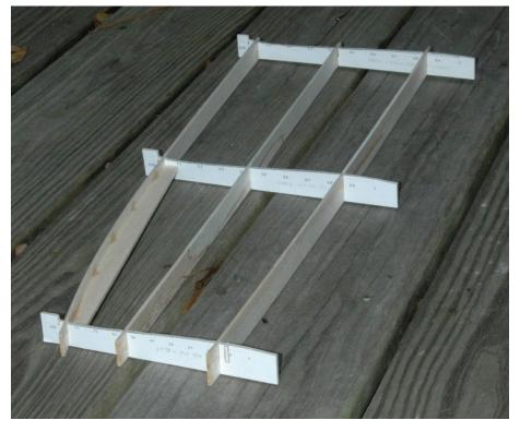
Figure W21: Tip panel jig
