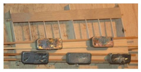
Figure W15: Clamping the top D-box skin in place
