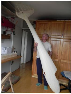
Above left: Fuselage in the making – gluing multilayer longitudinal battens Above: Fuselage is separated from assembly preparation
