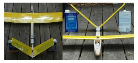
Figure F12: Gluing the tail pivot tubes to the fuselage
