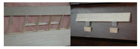
Figure W18: Spoiler frame, spoiler panel and hinge blocks
