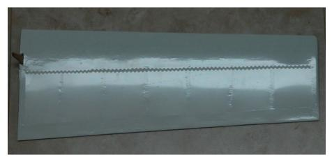
Figure T8: Tail panel with turbulator tape
