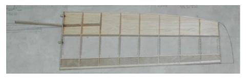
Figure W23: Tip panel frame ready for top D-box and trailing edge skins
