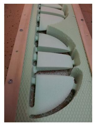
Wings finishing is milled threedimensionally from Styrodur
