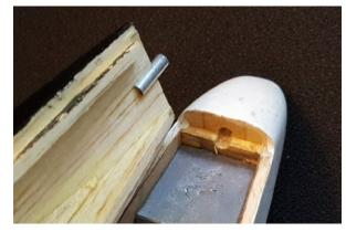
Figure F19: Hatch cover retaining pin
