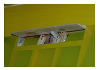
Figure W20: Installed spoiler with rubber band closing spring. Note that the servo wire is sealed with RTV where it enters the spoiler box.
