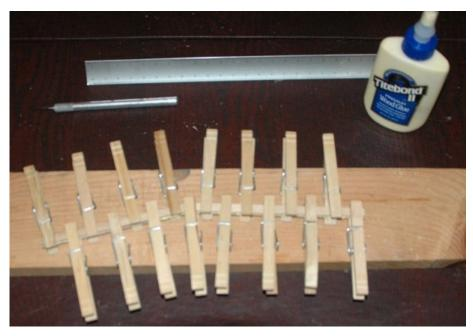
Figure W1: Laminating the tip joiner
