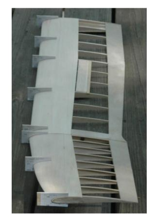
Figure W25: Wing with lots of leading edge templates
