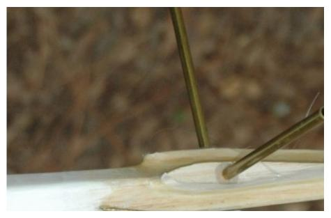
Figure F14: Tail Fairing Final Shaping and Glassing
