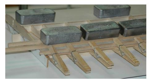
Figure W9: Clamping the trailing edge top skin
