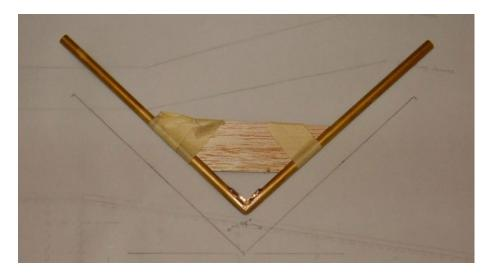
Figure T6: Tail pivot tube assembly template
