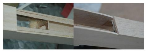
Figure F6: Applying fiberglass to the rear wing mount
