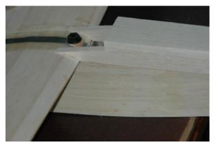
Figure F16: Fitting hatch cover to wing
