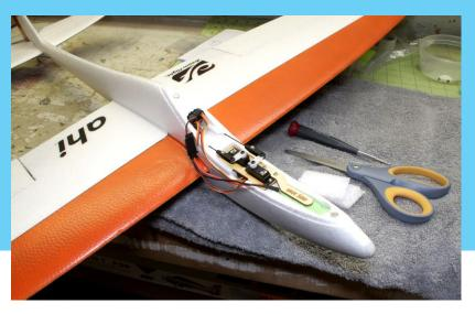
View showing the installed rudder and elevator servos, battery pack and battery hold-down.
