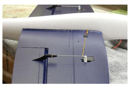
A close view of an installed aileron servo, linkage, and wiring.
