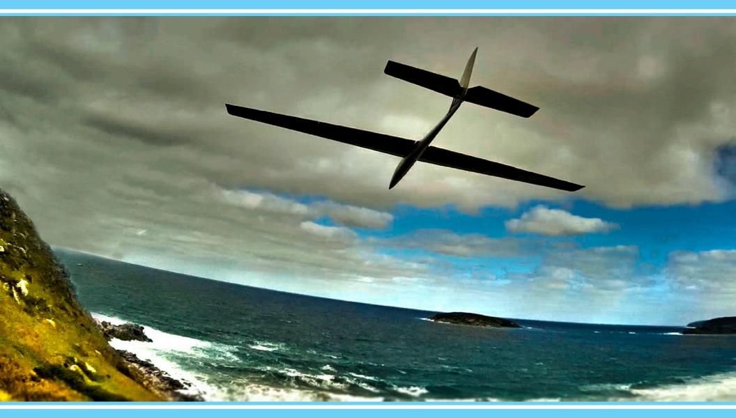
A Speedo flying at The Bluff, South Australia. This is a video grab from Adam Fisher's hat cam. The Speedo is sold by thebuildrc.com <a href="http://thebuildrc.com">http://thebuildrc.com</a>. The Speedo spans 1.4m and features balsa built-up wings with Oracover. Controls include ailerons and flaps, and it has a fiberglass fuselage.
