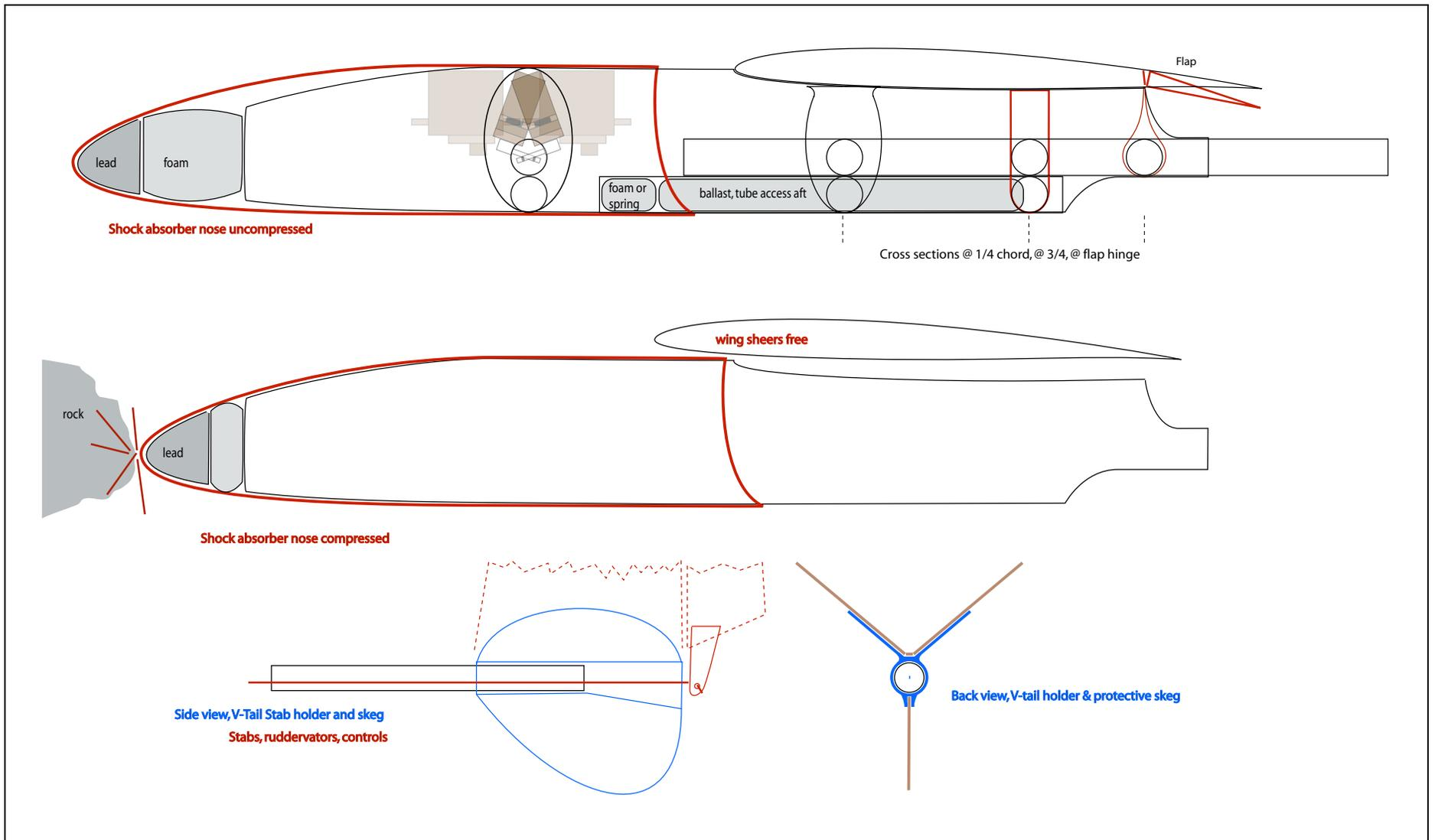
*Rock Bouncer fuselage with shock absorber nose cone and wing that shears free on impact. Not to scale. Serving suggestion only.*
