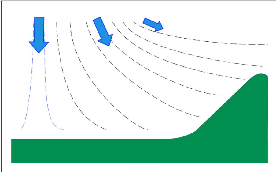
Illustration 4: Downdraft from collapsing thermal kills hill lift
