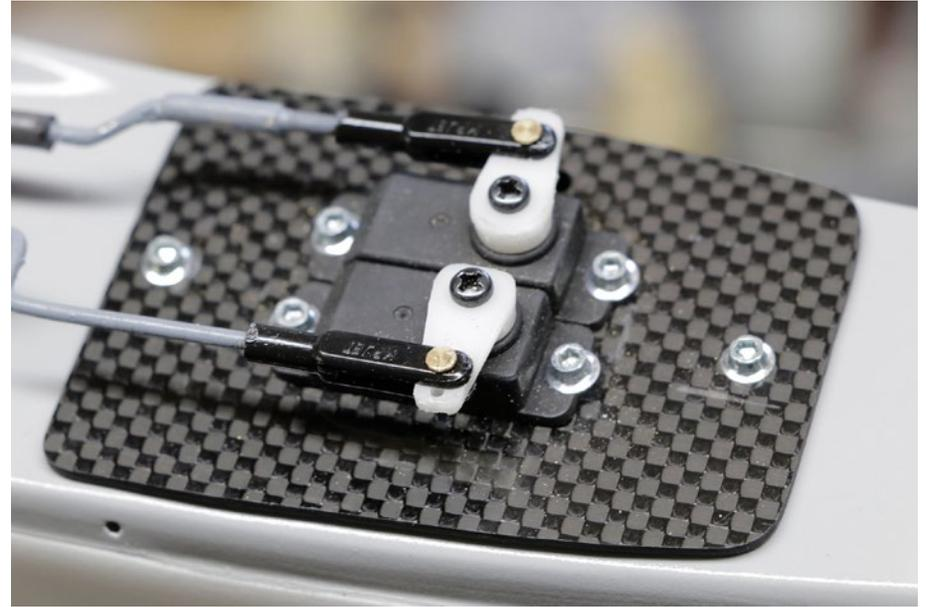
*I fabricated a new servo tray out of carbon plate to accommodate the small MKS servos and replaced one pushrod that had a fatal fracture in it. Notice the short servo arms to maximize the servo's resolution.*
