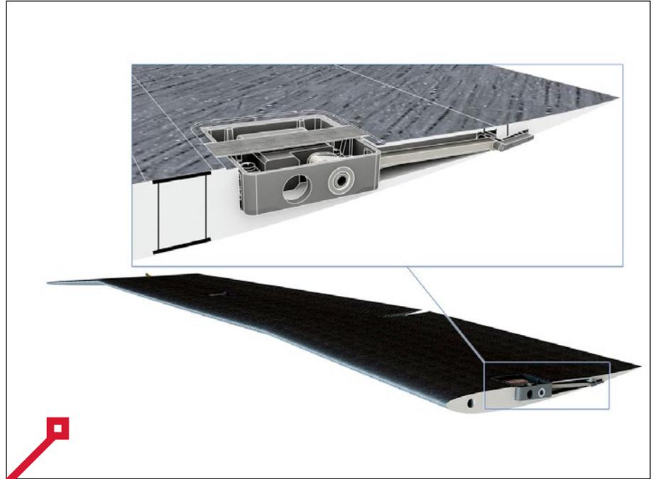
The wing comes with the IDS servo drive system already in place. The linkages for the center flap and inboard ailerons are all hidden inside the wing. No linkages are in the airstream.
