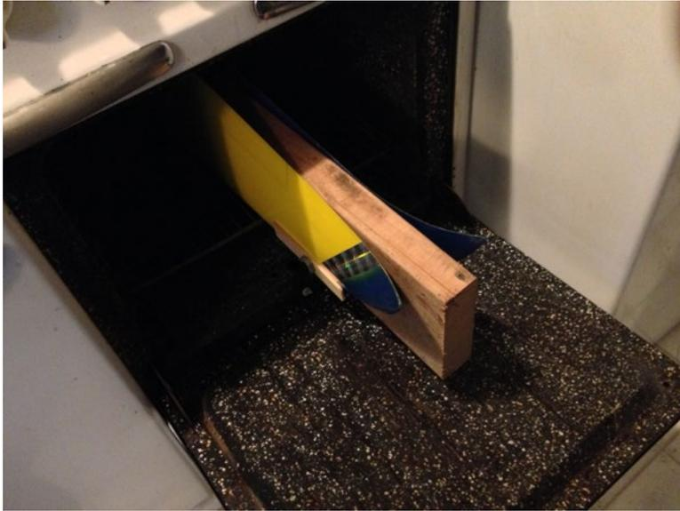
4: Putting the assembly into the oven on low heat.
