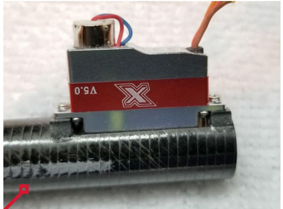
By using a round drive wheel with a pull cable, you wind up with linear servo output rather than output that changes as occurs with a servo arm and a pushrod. Notice the groove in the round servo wheel the pull wire sits in.
