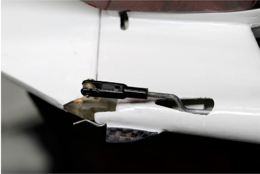
*On my model the tail skid which also secures the rudder keeper pin was missing completely. I fabricated a new tang and tail skid to hold the wire in place. Replaced the ancient nylon clevis with a MP jet fork which is much stronger.*
