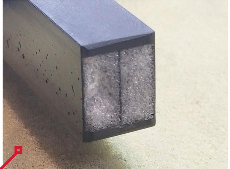
The joiner is rather unique. This allows the center wing panel, the A-tail booms and outer wing panel to all integrate into one single component, that is self-aligning and all the servos connect automatically. It is stronger than it looks.
