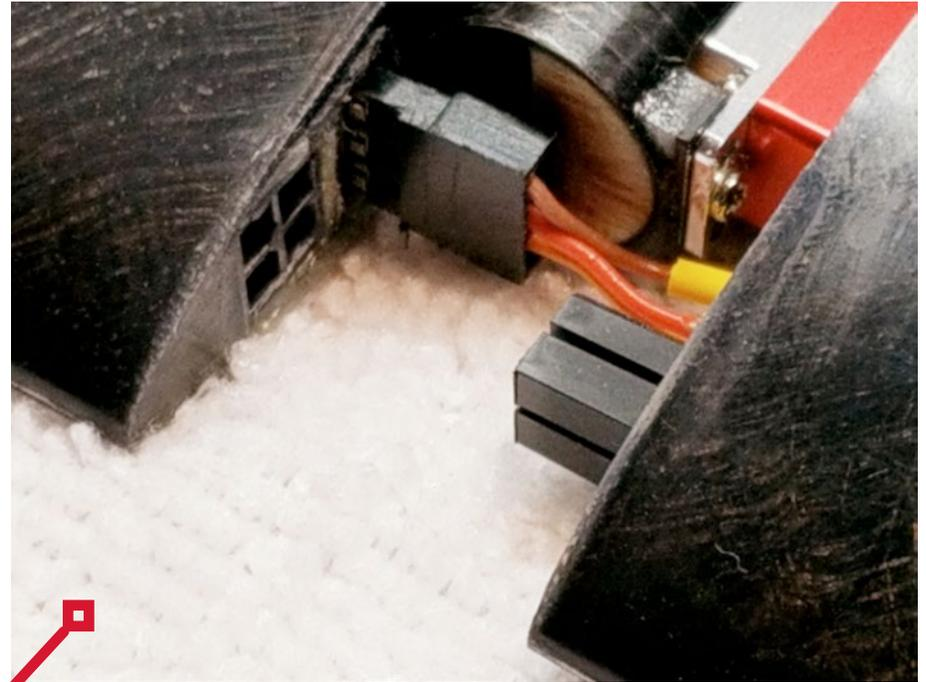
Electrical connections are already installed in the inboard and outboard panel which plug together automatically as the outboard wings lock in place.
