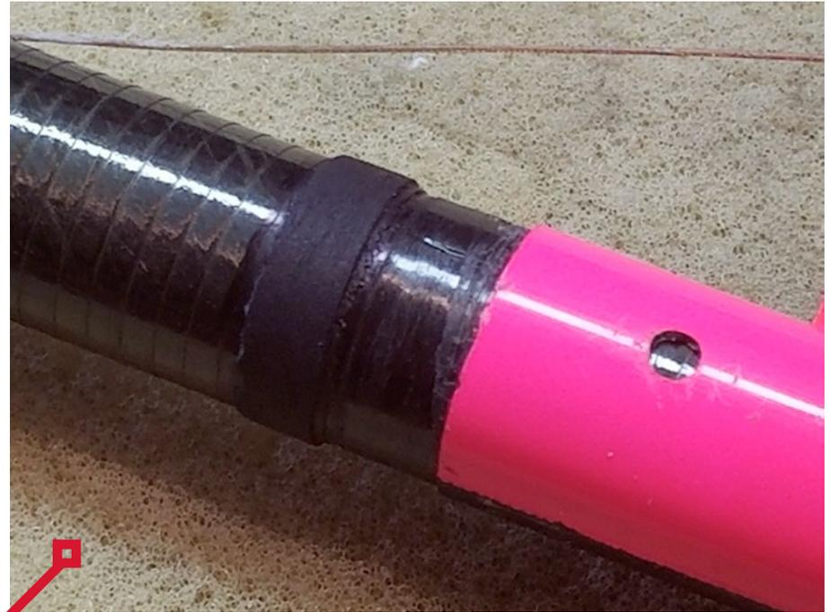
Start by covering with tape the area where you don't want the epoxy to bond to. Use a little water base jelly on the end and inside the tail where it slips over the boom.
