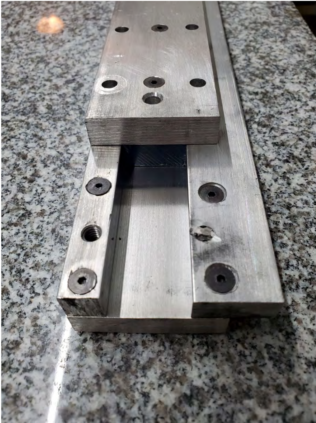
Blade spar jig end view. In use, the top and bottom would be aligned.
