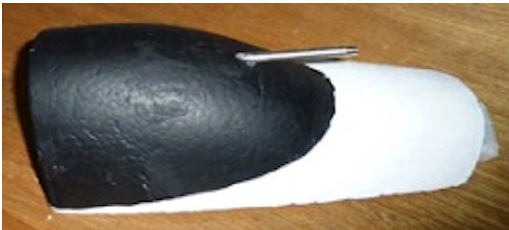
Photo 1: FrSky ASI installed in the canopy of an ageing Hobby King Bixler.
