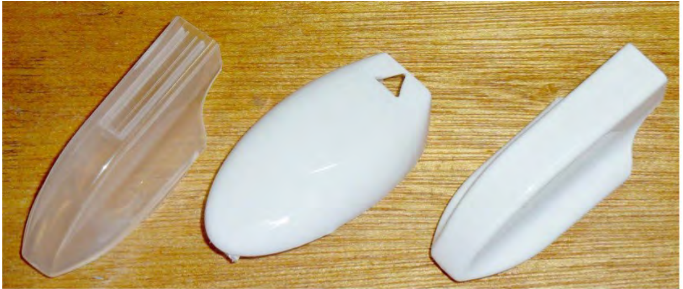
Photo 3: DIY servo arm fairings fashioned from discarded spray bottles.
