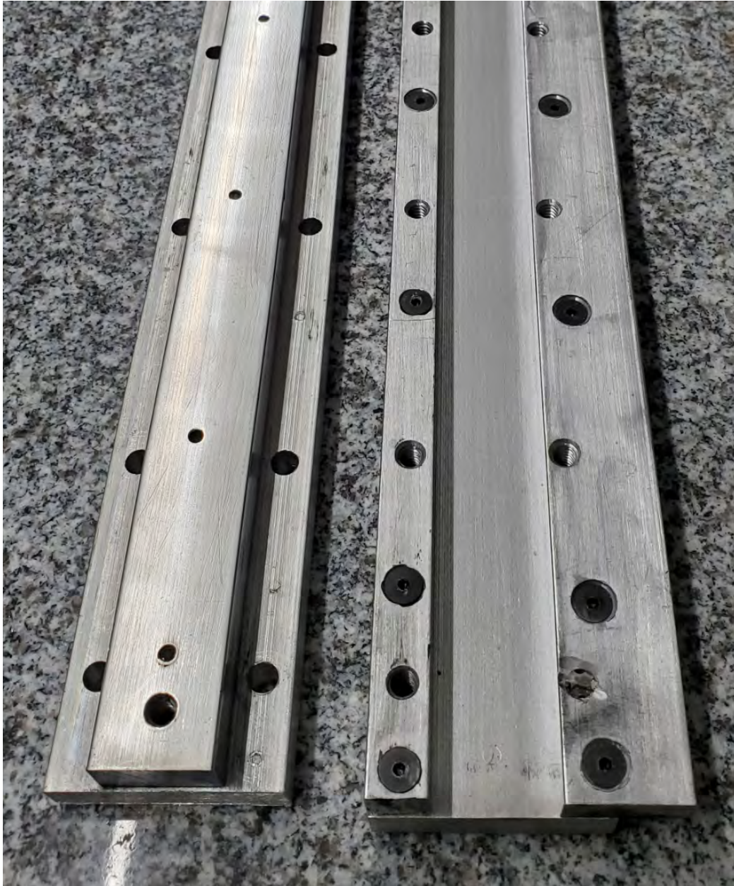
Aluminum blade jig made by the author.
