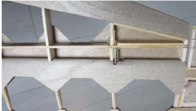
Left: stabiliser mounting strips and hinged control rod of the elevator. | Right: The hinge is in the 'locked' position. It will later be sheeted with ply.
