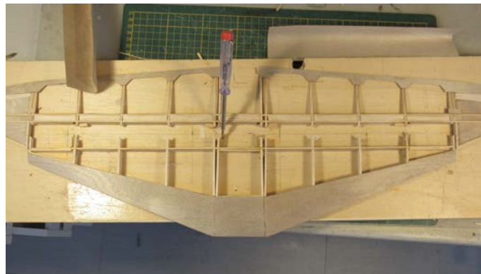
Left: devWing top view of stabiliser. | Right: Stabiliser roughly finished, elevator already cut loose.
