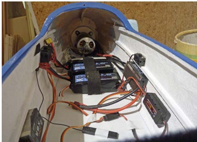
Left: The business end of the Javelot with the blanking plate fitted. | Right: Power train layout in the 'Super Javelot'.
