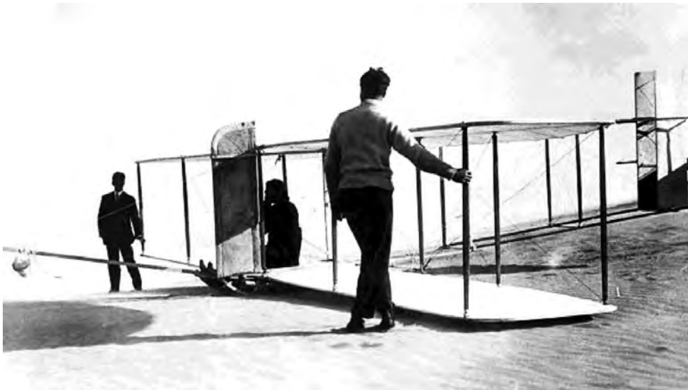
Lorin Wright (left) and Alec Ogilvie ready to lift the glider prior to hand launching. A bag of sand in the front counterbalanced the weight of the extended fuselage, counteracting the tail. (credit: Flugsport, November 29, 1911)
